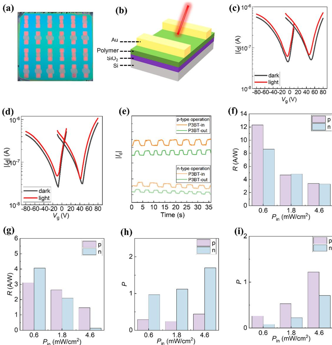
**Fig. 4** (a) Photograph of NIR OPTs. (b) The BG/TC device structure of NIR OPTs. (c) and (d) Transfer curves of the (c) P3BT-in and (d) P3BT-out NIR OPTs in the dark and under NIR light illumination (810 nm,  $4.6 \text{ mW cm}^{-2}$ ). (e) Photocurrent response upon the repeated optical on/off modulations of the NIR light. The responsivity ( $R$ ) and photo/dark current ratio ( $P$ ) under different light illumination (f) and (h) for P3BT-in (g) and (i) and P3BT-out.
