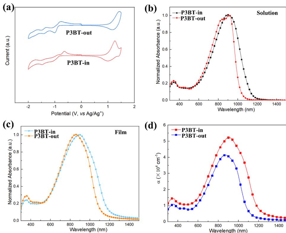
Fig. 2 (a) Cyclic voltammetry (CV) of polymer films; (b) and (c) UV-vis-NIR absorption spectra of P3BT-in and P3BT-out (b) in solution and (c) as films; (d) absorption coefficients ( $\alpha$ ) of the polymer thin films.
