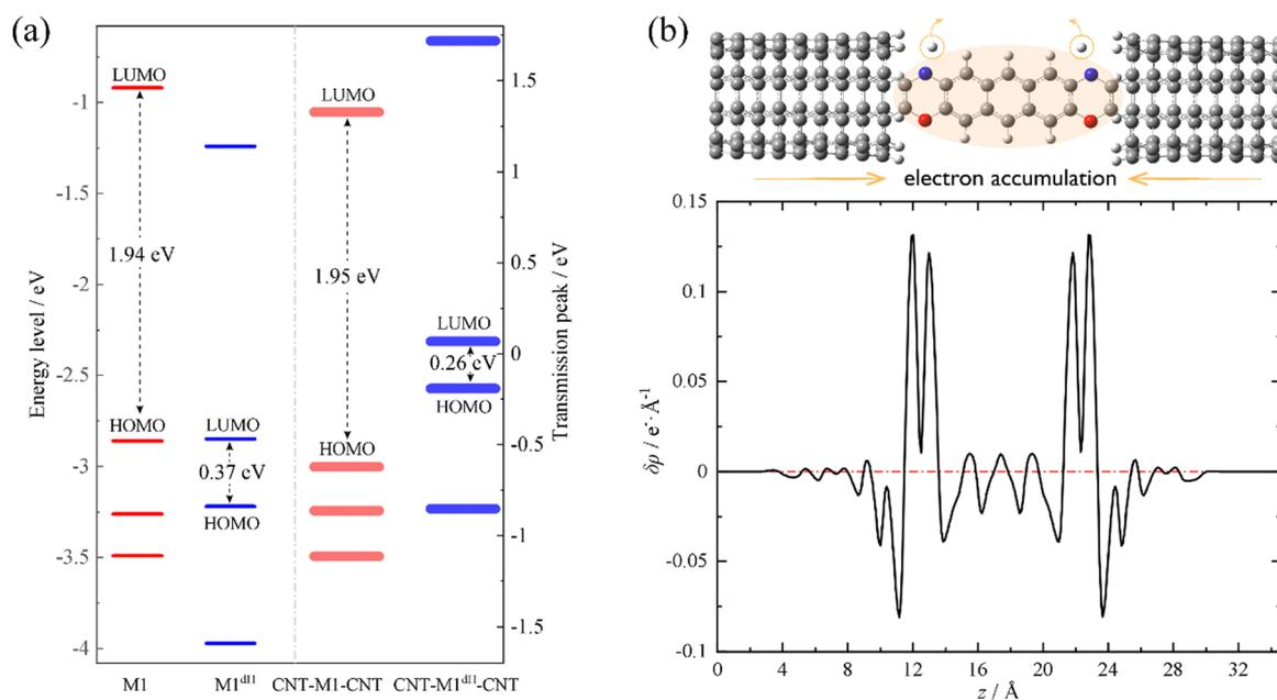
Fig. 2 (a) Molecular energy levels of the isolated M1 (red thin lines) and M1<sup>dH</sup> (blue thin lines) molecules, and the energy centers of the corresponding transmission peaks in the SWCNT-M1-SWCNT (red thick lines) and SWCNT-M1<sup>dH</sup>-SWCNT (blue thick lines) junctions. (b) The *xy*-plane averaged charge density difference  $\delta\rho(z)$  between the SWCNT-M1-SWCNT and SWCNT-M1<sup>dH</sup>-SWCNT junctions.
