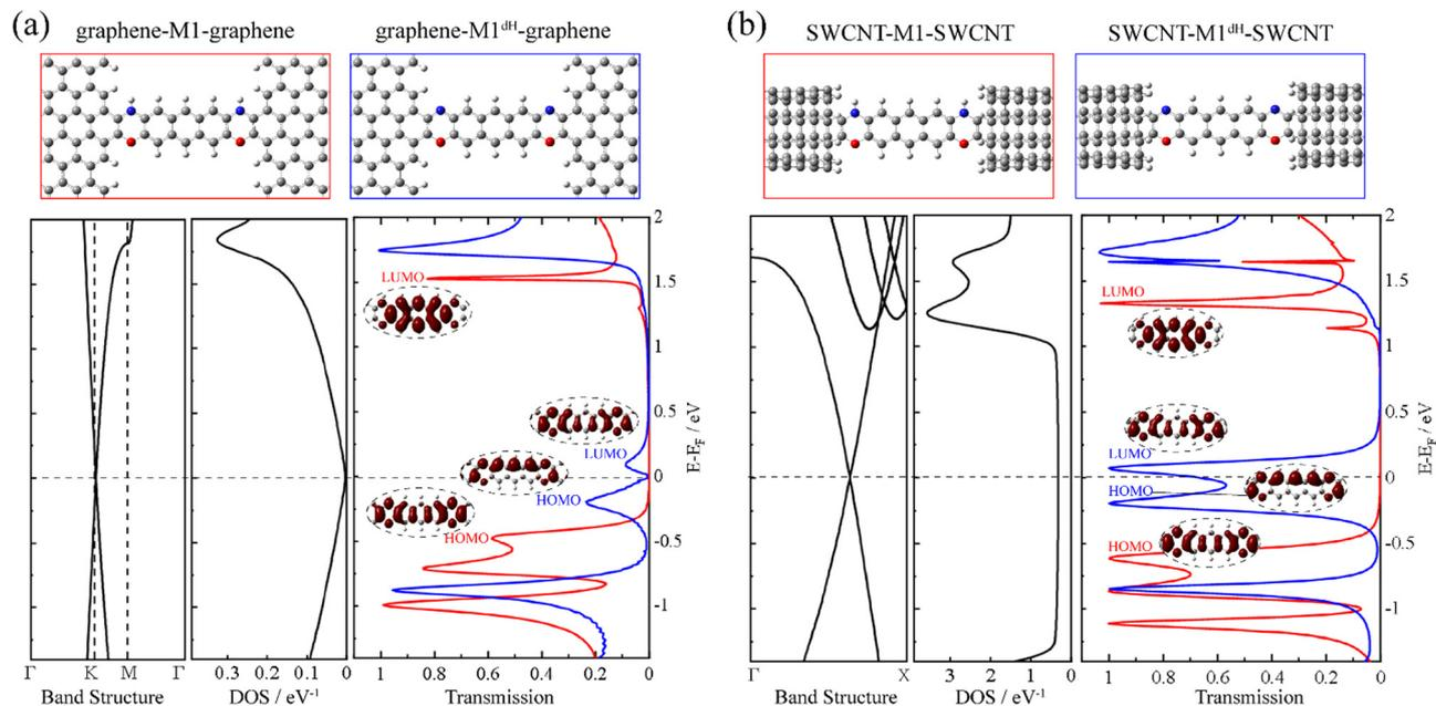
Fig. 1 The optimized atomic structures and the corresponding transmission spectra of graphene-M1-graphene (red line) and graphene-M1<sup>dH</sup>-graphene (blue line) in (a), and of SWCNT-M1-SWCNT (red line) and SWCNT-M1<sup>dH</sup>-SWCNT (blue line) in (b), together with the band structure and DOS of graphene in (a) and those of the (5,5) SWCNT in (b). The insets show the conducting eigenchannels for selected transmission peaks around  $E_F$ .
