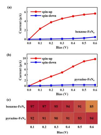
Fig. 6 Spin-resolved I-V curves of (a) SWCNT-benzene-FeN<sub>4</sub>-SWCNT-BS and (b) SWCNT-pyrazine-FeN<sub>4</sub>-SWCNT-BS. In panel (c), the calculated spin-filtering efficiency as a function of bias within the 0.1-0.6 V range
