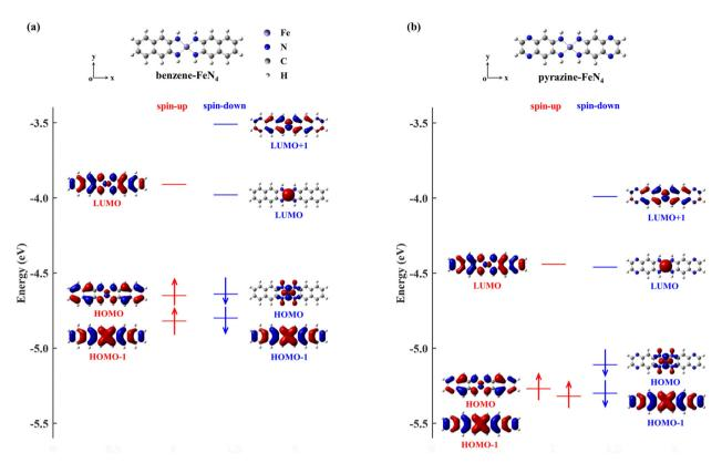
Fig. 2 Optimized atomic structure (the upper ball-and-stick diagrams), together with energy level arrangement and spatial distribution of the FMOs for isolated benzene $-FeN_4$  (a), and pyrazine $-FeN_4$  (b). Both benzene $-FeN_4$  and pyrazine $-FeN_4$  are placed in the x-y plane. Here, H, C, N, and Fe atoms are represented using the light grey, dark gray, blue and purple spheres, respectively.
