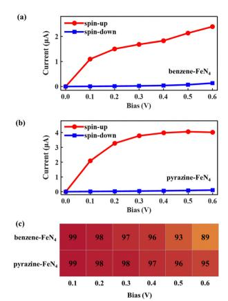
Fig. 4 Spin-resolved I-V curves of the SWCNT-benzene-FeN<sub>4</sub>-SWCNT junction (a) and the SWCNT-pyrazine-FeN<sub>4</sub>-SWCNT junction (b). (c) Calculated spin-filtering efficiency as a function of the bias voltage within the bias range of 0.1 to 0.6 V for the SWCNT-benzene-FeN<sub>4</sub>-SWCNT junction (the upper row), and the SWCNT-pyrazine-FeN<sub>4</sub>-SWCNT junction (the bottom row)
