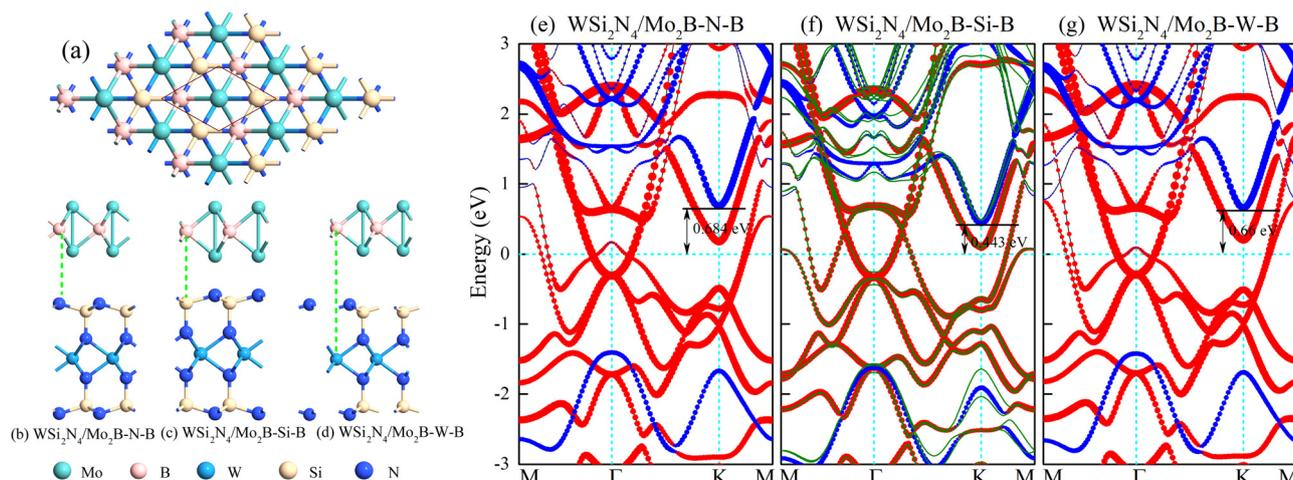
**Fig. 1** (a) and (b)–(d) Top view and side view of the structures of WSi<sub>2</sub>N<sub>4</sub>/Mo<sub>2</sub>B heterostructures. (e)–(g) Projected band structures of WSi<sub>2</sub>N<sub>4</sub>/Mo<sub>2</sub>B heterostructures in three different stacking models. The red and blue lines denote the contributions from Mo<sub>2</sub>B and WSi<sub>2</sub>N<sub>4</sub>, respectively. The green lines represent the band structures with SOC.
