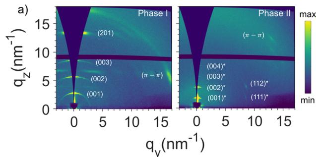
**Fig. 5** 2D GIWAXS patterns of p-DTS(FBTTh<sub>2</sub>)<sub>2</sub> phase I (a) and phase II (b), for comparison.
