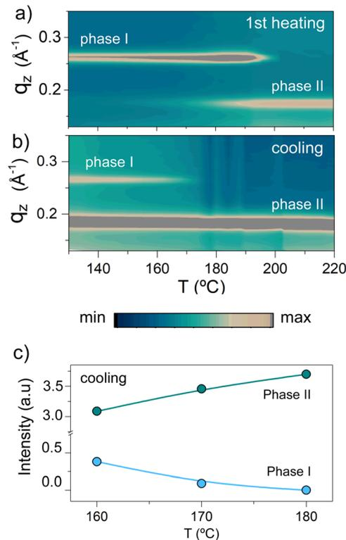
**Fig. 4** (a) Azimuthally integrated GIWAXS intensity recorded during heating (upper panel) and cooling (lower panel) at approximately 20 °C min<sup>-1</sup> for p-DTS(FBTTh<sub>2</sub>)<sub>2</sub> confined in 60 nm pores. (b) Evolution of the intensity of the characteristic reflection peaks of phase I and phase II during cooling.
