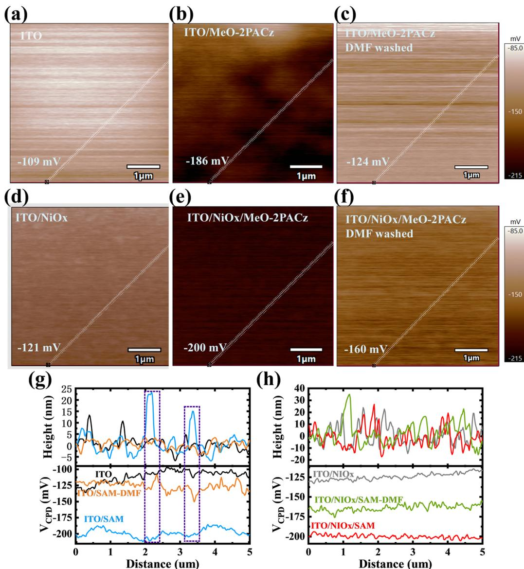
Fig. 2 KPFM images of ITO (a) without and (b) with MeO-2PACz modification, and (c) further washed by DMF. KPFM images of ITO/NiO<sub>x</sub> (d) before and (e) after MeO-2PACz modification, and (f) washed by DMF. (g) and (h) The potential and height variation diagram along the white lines on different substrates.
