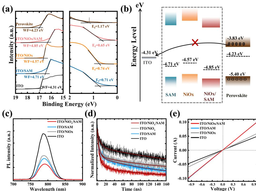
Fig. 4 (a) UPS spectra of the ITO, ITO/SAM, ITO/NiO<sub>x</sub>, ITO/NiO<sub>x</sub>/SAM and perovskite. (b) Energy level diagram of PSCs. (c) PL and (d) TRPL measurement results of the perovskite films on the different substrates. (e) DC conductivity of the ITO, ITO/SAM, ITO/NiO<sub>x</sub> and ITO/NiO<sub>x</sub>/SAM films.
