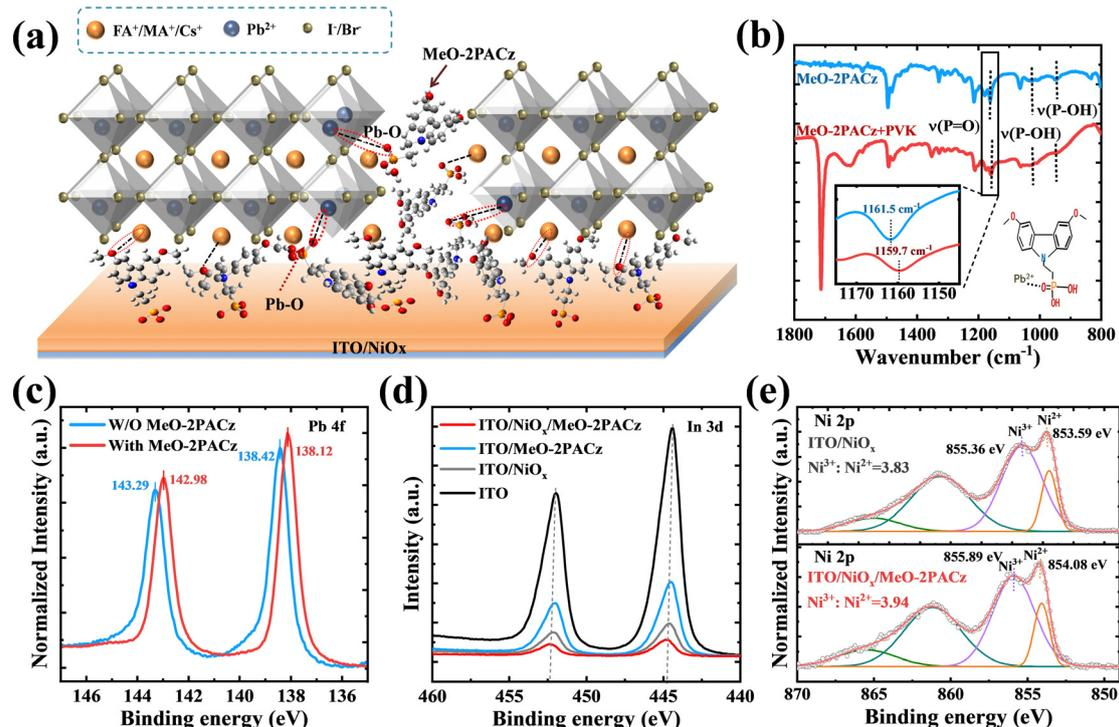
Fig. 3 (a) Schematic diagram of bottom interface defect passivation of PVK by MeO-2PACz molecules anchored on NiO<sub>x</sub>. (b) FTIR spectra of MeO-2PACz, and the MeO-2PACz + PbI<sub>2</sub> complex. (c) XPS spectra of Pb 4f for the perovskite films with or without MeO-2PACz modification. The XPS of (d) the In 3d region of ITO and ITO/NiO<sub>x</sub> and (e) the Ni 2p region of ITO/NiO<sub>x</sub> before and after the adsorption of MeO-2PACz.
