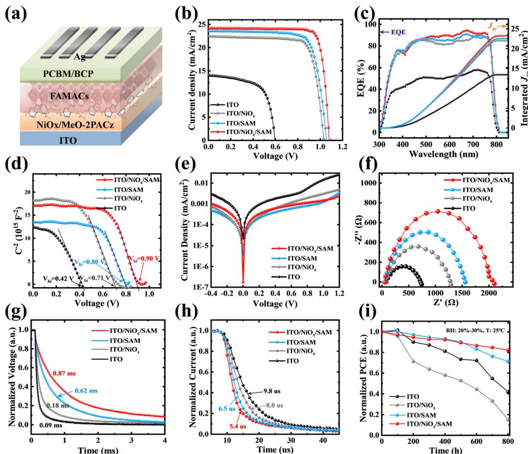
Fig. 5 (a) Device structure diagram based on NiO<sub>x</sub>/SAM. (b)  $J$ - $V$  curves and (c) EQE measurement results for four different devices. (d) Dark  $J$ - $V$  measurements of the PSC devices. (e) The transient photovoltage (TPV) decay curve and (f) transient photocurrent (TPC) decay curve. (g) Mott-Schottky analysis. (h) EIS curves of PSC devices. (i) The stability of the devices at 25 °C and RH = 30%.
