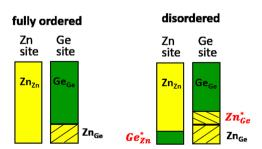
Fig. 1 Schematic of the cation occupation of the two cation sites of the β-NaFeO<sub>2</sub> structure type. The left-hand case has no intrinsic disorder and a certain degree of extrinsic disorder ( $Zn_{Ge}$ ), while the right-hand case depicts the same composition with extrinsic ( $Zn_{Ge}$ ) and intrinsic ( $Zn_{Ge}^*$  and
