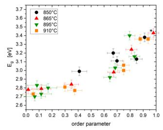
Fig. 11 Order parameter *versus* optical bandgap  $E_{\alpha}$ . The star marks the  $Zn_{1+x}Ge_{1-x}(N_{1-x}O_x)_2$  compound with nearly full cation order.
