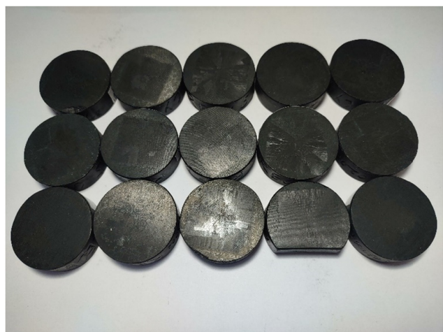
Fig. 7 Recycled YBCO bulks. One bulk was cut due to the presence of secondary grains. The bulks were marked with letters A–O. From left to right, in the first row are bulks A–E, in the second row are bulks F–I and in the third row are bulks H–O.
