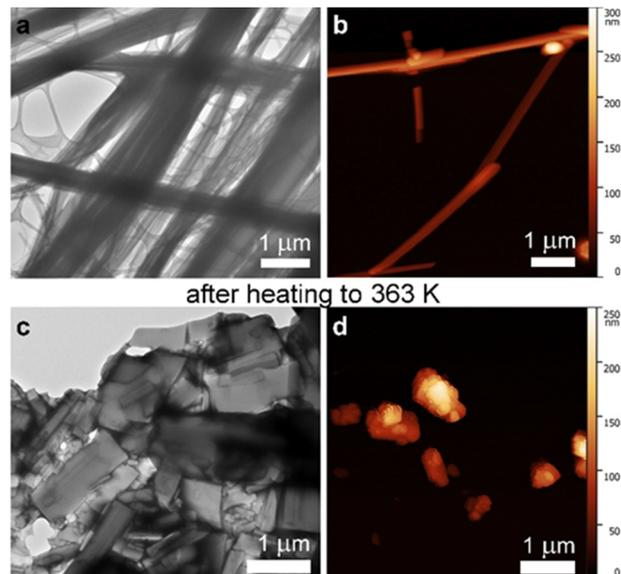
Fig. 5 TEM (a) and (c) and AFM (b) and (d) micrographs of the heterochiral tetrapeptide forming fibrils at rt (a) and (b) which irreversibly converted into plates upon heating to 363 K (c) and (d).
