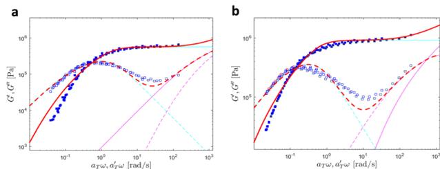
Fig. 19 Linear viscoelastic mastercurves of (a) PBA-U8 and (b) PBA-U13 at  $T_{ref} = 40$  °C. Red lines correspond to the model predictions obtained with the values shown in Tables 1 and 2. The contributions of the Rouse model (in magenta) and the slow modes (in cyan) are also presented.
