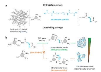
Fig. 1 Synthetic strategy of DGL G5-PEG hydrogels. (a) Schematic representation of hydrogel precursors, DGL G5 dendrigrafts and dicarboxylic acid-PEG polymers. (b) Crosslinking reaction based on intermolecular amide bonds (network crosslinks) formation between the DGL G5 nanoparticles. Increasing DGL G5 concentration (intermolecular proximity) in the hydrogel precursor solution favours the formation of intermolecular amide bonds (network crosslinks)
