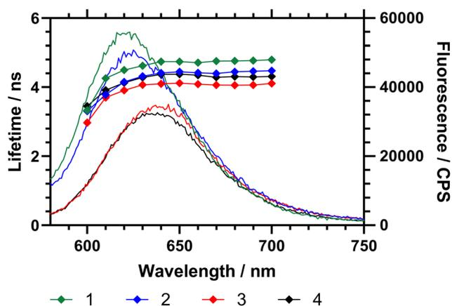
Fig. 6 Fluorescence emission spectra (15 °C) of HB-P(NIPAM-co-NR)-VAN polymers with emission spectra (left axis) and emission wavelength specific excited state lifetime (right axis).  $\lambda_{ex} = 570$  nm. Polymer 1 (DB 0.107) is black (◆); 2 (DB 0.065) is red (◆); 3 (DB 0.044) is blue (◆).
