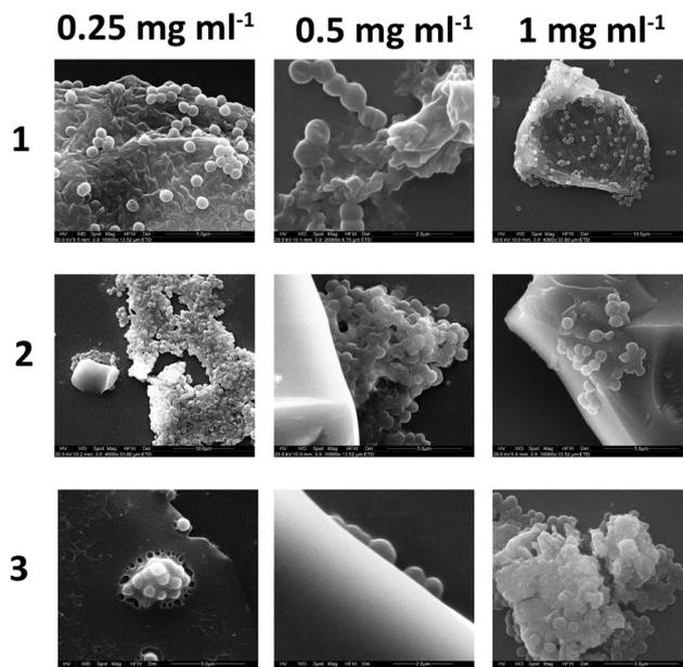
Fig. 10 SEM images of combined 10<sup>8</sup> cfu *S. aureus* + HB-PNIPAM-Vanc solutions dried on a glass plate.
