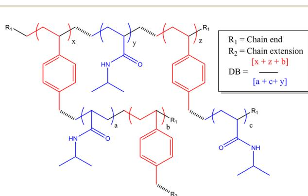
Scheme 1 Chemical structure of **HB-PNIPAM-VAN** polymer backbone.
