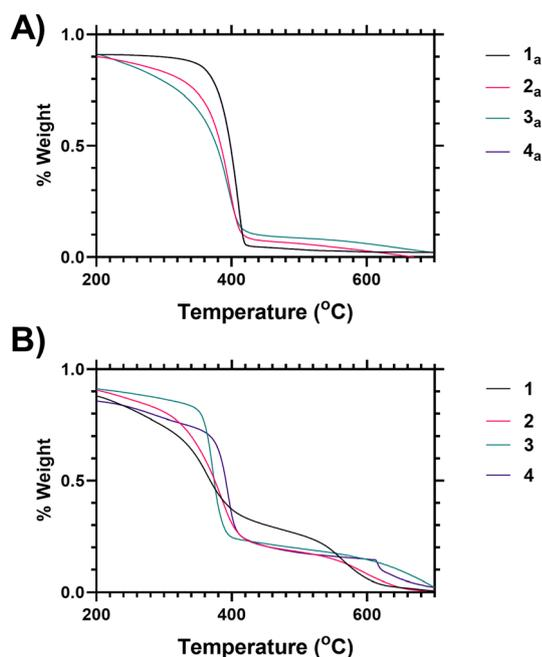
Fig. 1 (A) Thermogravimetric analysis (TGA) mass loss profiles for polymers 1–4 (B) TGA analysis for precursor polymers 1<sub>a</sub>–4<sub>a</sub> (unmodified pyrrole/acid chain ended products of SCVP RAFT synthesis process prior to chain end modification).
