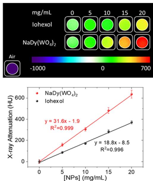
Fig. 9 X-ray attenuation phantom images (top) and X-ray attenuation values in Hounsfield units (HU) (bottom) obtained for aqueous suspensions having different concentrations of NaDy(WO<sub>4</sub>)<sub>2</sub> NPs and iohexol.
