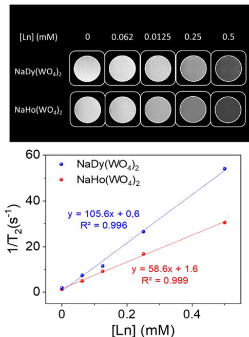
Fig. 6  $T_2$ -weighted phantom images (top) and relaxation rates ( $1/T_2$ ) vs. Ln concentrations (down) obtained at 9.4 T for aqueous suspensions of  $\text{NaDy}(\text{WO}_4)_2$  (blue) and  $\text{NaHo}(\text{WO}_4)_2$  (red) NPs.
