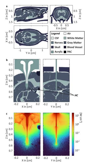
**Fig. 2** MS Simulation. (a) Rat head model segmented into six different kinds of tissue; (b) head section and probe in HC with; (c) heatmap depiction of the irradiance within the head section for 460 nm.‡
