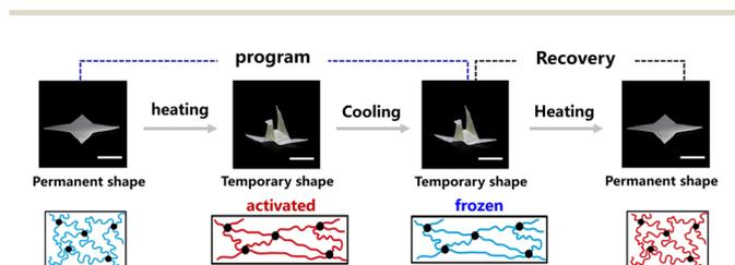
**Fig. 11** Demonstration of typical thermally induced shape memory effect. The upper parts show the sequentially changing structures and treatment during the process, and the bottom parts show the status of the chain mobility corresponding to each shape. The black round dots indicate the crosslinked points of the network, the blue lines indicate the polymer chains with the mobility frozen and the red lines indicate the polymer chains with the mobility activated.
