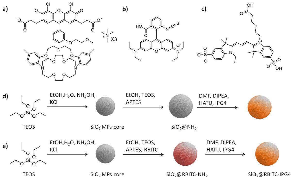
**Fig. 1** Molecular structure of the employed dye and synthetic scheme for the synthesis of silica microsensors: (a) molecular structure of IPG4 TMA salt; (b) molecular structure of rhodamine B isothiocyanate; (c) molecular structure of cyanine 3; (d) synthesis scheme with reaction conditions of  $\text{SiO}_2\text{@IPG4}$ ; and (e) synthesis scheme with reaction conditions of  $\text{SiO}_2\text{@RBITC-IPG4}$ .
