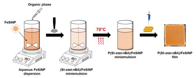
Scheme 1 Schematic diagram showing the nanocomposite film preparation strategy, starting with polymer nanocomposite latex synthesis by miniemulsion polymerisation, followed by drop casting to prepare a film.
