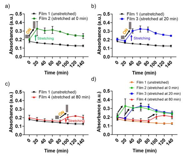
Fig. 6 On-demand activation of peroxidase enzyme-mimicking activity by stretching the P(St-stat-nBA)/FeSiNP (10 wt%) films at different time points: (a) 0 min, (b) 20 min, (c) 80 min; (d) plot showing combined stretching effects at different time points.
