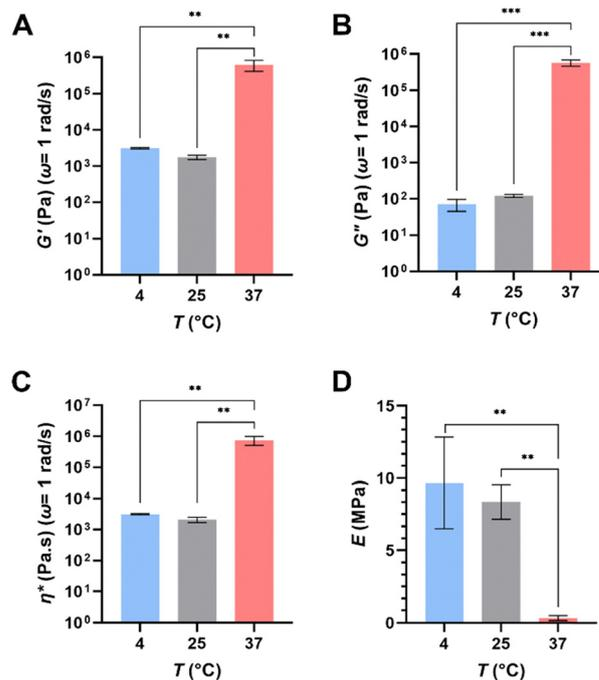
Fig. 5 Results of rheological and compression testing of cross-linked hydrogels printed using the final chosen formulation. (A) Quantification of the storage moduli,  $G'$ , (B) loss moduli,  $G''$ , (C) complex viscosity,  $\eta^*$  and (D) compressive (Young's) moduli,  $E$ , of hydrogels at three different temperatures. All results reported for at least  $n = 3$ . \*\*  $p \leq 0.01$ , \*\*\*  $p \leq 0.001$ .
