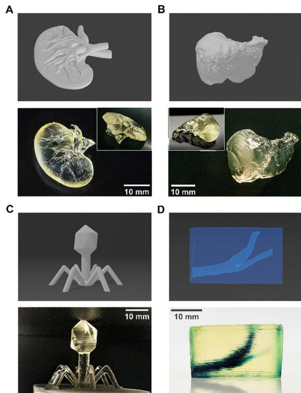
**Fig. 9** The photoink can print a range of different structures at high print fidelity – STL files vs. actual prints. (A) Miniature human kidney (inset: reverse); (B) miniature human liver (inset: ventral view); (C) enlarged bacteriophage virus; (D) hollow structure with human carotid (contains blue food dye for visibility; see ESI,† Video V1). All scale bars = 10 mm.
