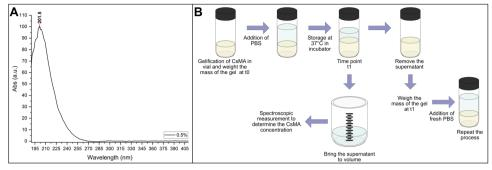
Fig. 3 (A) UV-vis spectra of a 0.5% water solution of CsMA; the maximum absorbance was detected at 201.5 nm. To avoid signal saturation, the intensity was measured at 215 nm. (B) Methodology to determine the amount of CsMA released into the PBS solution (solubilization), and the amount of CsMA hydrogel broken in smaller pieces and removed at each time point (degradation).
