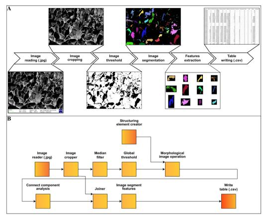
Fig. 2 (A) Pore analysis of SEM images and an automated procedure. Forty images were collected at 1000× magnification, cropped, thresholded and segmented. Once segmented, the features were extracted, and the dimension and shape parameters calculated. (B) Implemented workflow using Knime showing the used nodes.
