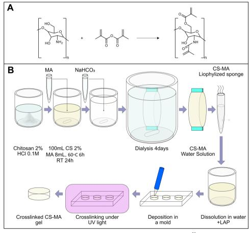
Fig. 1 (A) The proposed chemical reaction is extrapolated from previous works in the literature.<sup>25</sup> The added methacrylic groups allow the photocrosslinking of the solution to form a hydrogel. (B) Preparation of CsMA stock and successive preparation of CsMA crosslinked hydrogels.
