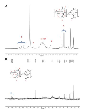
Fig. 5 (A)  $^{1}\text{H-NMR}$  NMR of chitosan–methacrylate. (B)  $^{13}\text{C-NMR}$  NMR of chitosan–methacrylate.
