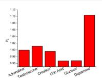
Fig. 9 Selectivity test: normalized emission response ( $I/I_0$ , where I and  $I_0$ are the emission intensities of the nanoparticles at 437 nm,  $\lambda_{exc}$  380 nm, after and before the addition of the analytes, respectively) of CNPs\_ART towards dopamine (0.1  $\mu M$  in water) over interfering analytes (1  $\mu M$  in water, pH 7).
