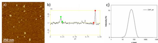
Fig. 3 (a)  $1 \times 1 \mu\text{m}^2$  AFM height image of CNPs\_ART, the height scale is 5 nm; (b) exemplificative cross-sections, used for the determination of the nanoparticle height; (c) particle size distribution of CNPs\_ART ( $1 \text{ mg mL}^{-1}$ ) in water at  $25 \text{ }^\circ\text{C}$ .
