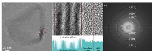
Fig. 4 (a) C-TEM image of CNPs\_ART; (b) C-TEM magnified image of the black box in (a) with its relative intensity profile (lower panel), showing the multilayer structure of CNPs\_ART with an interplanar distance of  $0.339 \pm 0.03 \text{ nm}$  and the amorphous carbon coating on its surface; (c) FFT image of (a) with indexed CNP's atomic planes.
