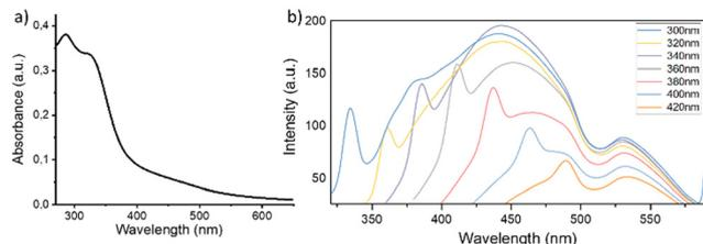
Fig. 6 (a) UV-vis spectrum of CNPs\_ART (0.05 mg mL<sup>-1</sup> in MilliQ water). (b) Fluorescence emission spectra of CNPs\_ART (0.05 mg mL<sup>-1</sup> in MilliQ water, pH 7) at different excitation wavelengths (from 300 to 420 nm, see the inset).
