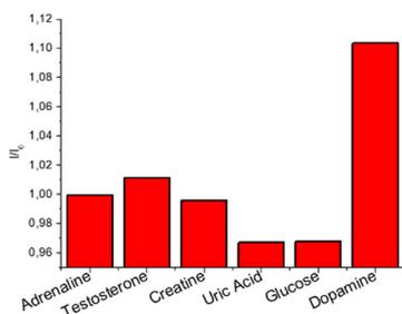
Fig. 9 Selectivity test: normalized emission response ( $I/I_0$ , where  $I$  and  $I_0$  are the emission intensities of the nanoparticles at 437 nm,  $\lambda_{\text{exc}}$  380 nm, after and before the addition of the analytes, respectively) of CNPs\_ART towards dopamine (0.1 μM in water) over interfering analytes (1 μM in water, pH 7).
