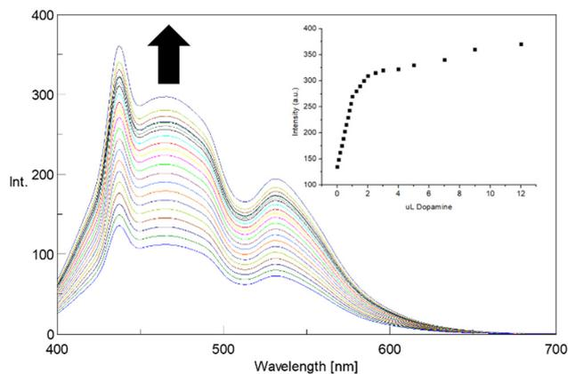
Fig. 7 Fluorescence emission spectra of CNPs\_ART solution (0.01 mg mL<sup>-1</sup> in MilliQ water,  $\lambda_{\text{ex}} = 380$  nm) upon addition of DA (0–12 μM). Inset shows the calibration curve.
