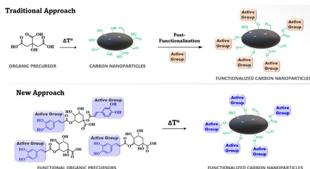
Fig. 2 Schematic representation of two different synthetic approaches.
