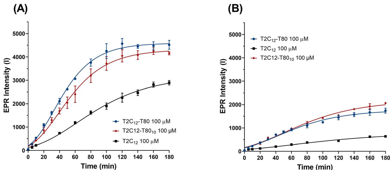
Fig. 4 (A) EPR enzymatic assays with  $12 \text{ U mL}^{-1}$  of CE2 in the presence of T2C<sub>12</sub> 100 μM, T2C<sub>12</sub>-T80<sub>10</sub> 100 μM and T2C<sub>12</sub>-T80 100 μM. (B) Enzymatic assays of T2C<sub>12</sub> 100 μM, T2C<sub>12</sub>-T80<sub>10</sub> 100 μM and T2C<sub>12</sub>-T80 100 μM with CE1  $12 \text{ U mL}^{-1}$ . All kinetics were performed at 37 °C with stirring at 400 rpm, and the continuous line was drawn to better show the course of the points.
