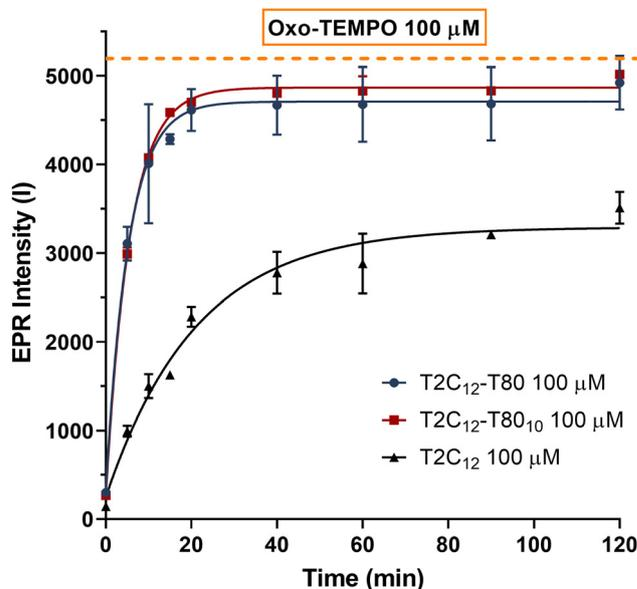
Fig. 3 EPR enzymatic assays with 0.5 U mL<sup>-1</sup> of PLE in the presence of T2C<sub>12</sub> 100 μM, T2C<sub>12</sub>-T80<sub>10</sub> 100 μM or T2C<sub>12</sub>-T80 100 μM micelles maintained at 37 °C under stirring at 400 rpm. The continuous line is drawn to better show the course of the points.
