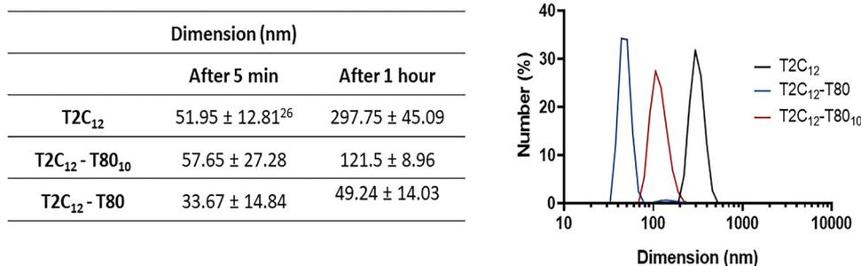
Fig. 2 (left) Table with hydrodynamic diameters of T2C<sub>12</sub> 100 μM, T2C<sub>12</sub>-T80<sub>10</sub> 100 μM and T2C<sub>12</sub>-T80 100 μM measured via DLS 5 min and 1 hour after the sonication step. (right) Number-weighted average size determined for T2C<sub>12</sub> 100 μM, T2C<sub>12</sub>-T80<sub>10</sub> 100 μM and T2C<sub>12</sub>-T80 100 μM micelles via DLS measurement after 1 hour from the sonication step.
