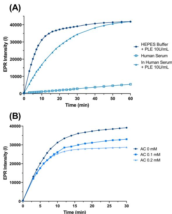
Fig. 8 Stability assessment with T2C<sub>12</sub>-T80 2 mM. (A) Incubation of the micelle probe HS and enzymatic kinetics with PLE 10 U mL<sup>-1</sup> in HEPES-buffered saline solution or in human serum. (B) Enzymatic kinetics with PLE 10 U mL<sup>-1</sup> in the absence and presence of ascorbic acid of 0.1 and 0.2 mM. All the assays were performed at room temperature.
