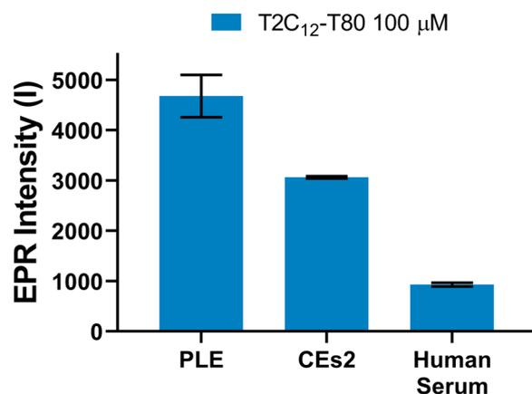
Fig. 6 EPR intensity detected upon 1 h incubation of T2C<sub>12</sub> 100 μM + T80 20 μM with PLE, CE2 and human serum at 37 °C under stirring at 400 rpm.
