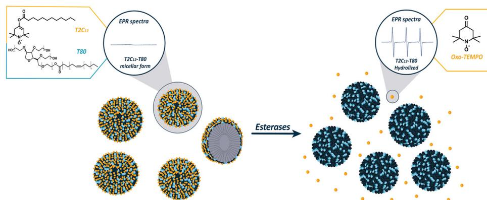
Fig. 1 Schematic representation of the EPR silent T2C<sub>12</sub>-T80 probe in the micellar form, followed by hydrolyzation in the presence of esterases and release of oxo-TEMPO, which display an intense EPR signal.
