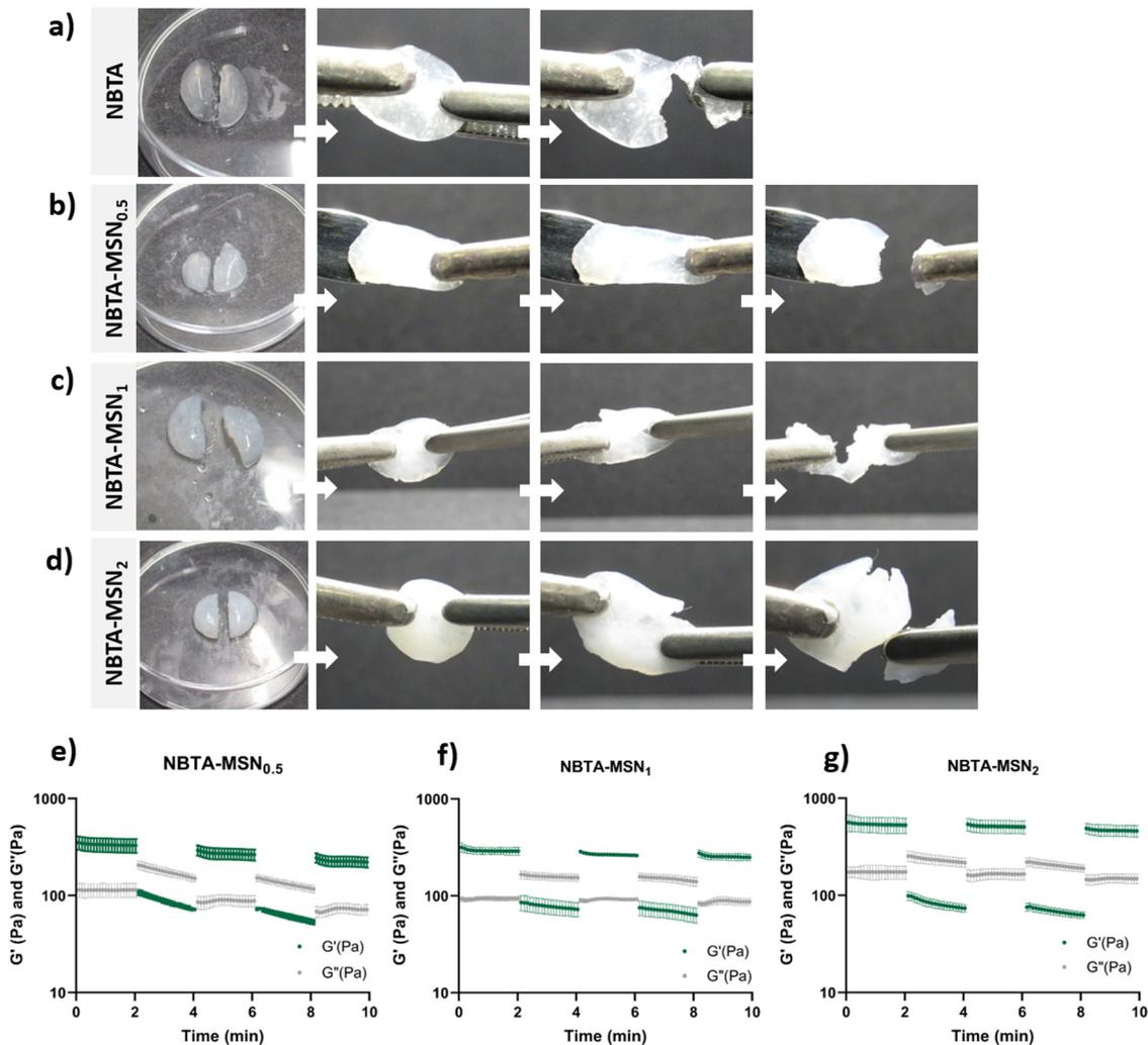
Fig. 5 Self-healing behaviour of NBTA-MSN hydrogels. Macroscopic self-healing test of (a) NBTA hydrogels, (b) NBTA-MSN<sub>0.5</sub>, (c) NBTA-MSN<sub>1</sub>, (d) NBTA-MSN<sub>2</sub>. Rheological self-healing test of (e) NBTA-MSN<sub>0.5</sub> gels, (f) NBTA-MSN<sub>1</sub> gels, (g) NBTA-MSN<sub>2</sub> gels.
