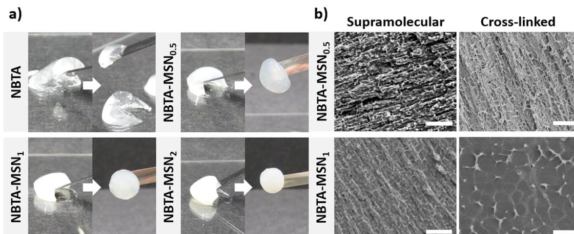
Fig. 3 Structural analysis of NBTA-MSN nanocomposites. (a) Optical images of NBTA-MSN hydrogels with various concentrations of MSNs. (b) Cryo-SEM images of NBTA-MSN<sub>0.5</sub> (scale bar: 5 μm) and NBTA-MSN<sub>1</sub> (scale bar: 5 μm before UV exposure, and 1 μm for after UV exposure) before and after MSN crosslinking upon UV exposure.
