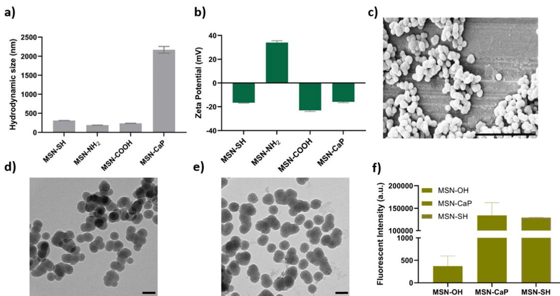
**Fig. 2** Characterization of the synthesized MSNs. (a) Hydrodynamic size of synthesized MSNs; (b) zeta potential of MSNs; (c) SEM imaging of MSN-SH (scale bar: 1  $\mu$ m); (d) TEM imaging of MSN-SH; and (e) MSN-CaP (scale bar: 50 nm); (f) ATTO647N-maleimide labeling of control particles (MSN-OH), MSN-SH and MSN-CaP.
