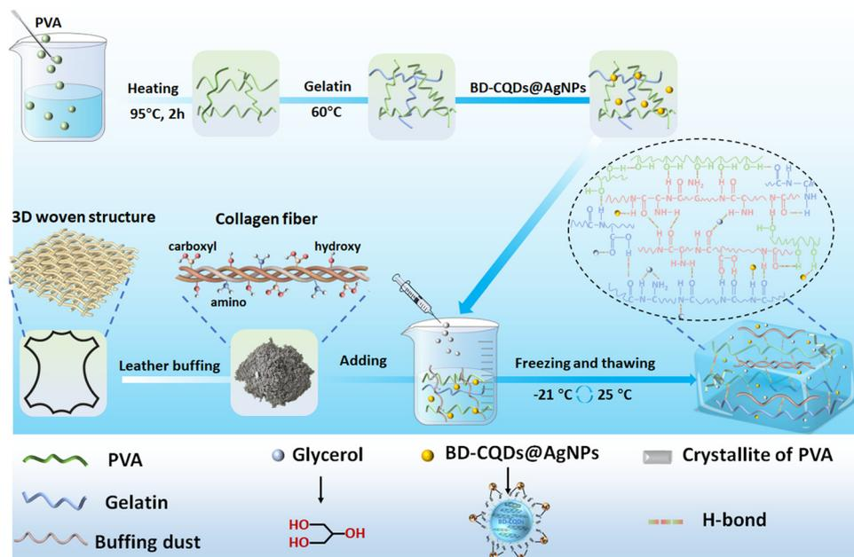
Fig. 1 Schematic fabrication route for the BPGC-Gly organohydrogel.
