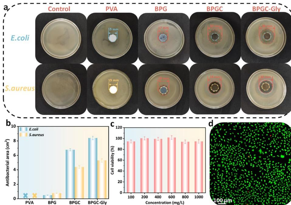
Fig. 4 Antibacterial and cytotoxicity properties of BPGC-Gly. Antibacterial pictures (a) and statistics of the antibacterial area (b) of PVA, BPG, BPGC, and BPGC-Gly against *E. coli* and *S. aureus*. (c) Cell viability of BPGC-Gly at different concentrations. (d) CLSM image of L929 cells after culturing for 24 h with 1000 mg mL<sup>-1</sup> BPGC-Gly extract (living cells: green fluorescence, dead cells: red fluorescence).
