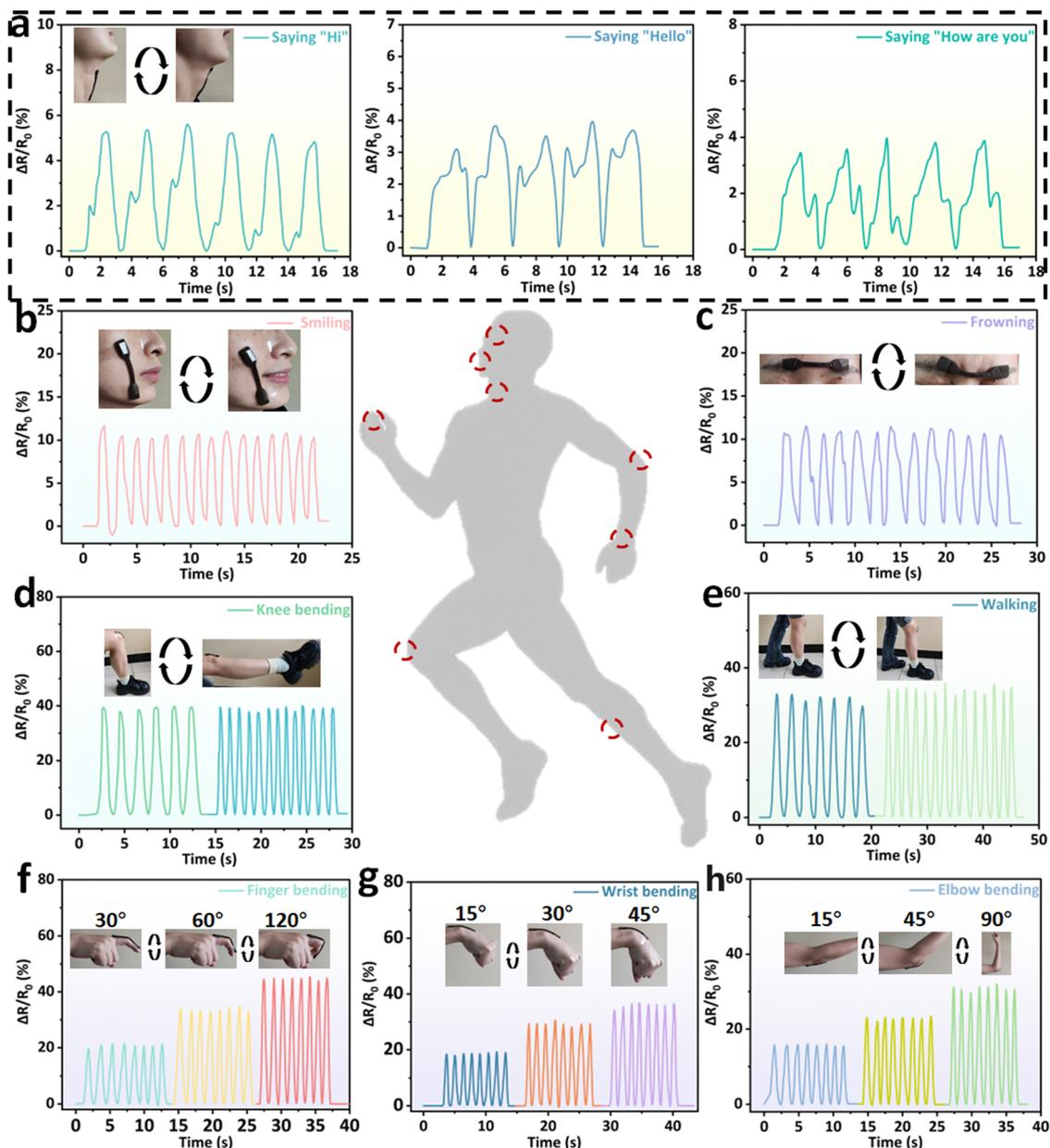
Fig. 7 Strain sensing property of the BPGC-Gly sensor. Real-time  $\Delta R/R_0$  change curves of BPGC-Gly as strain sensors to monitor various human movements, including human pronunciation (a), smiling (b) and frowning (c), knee bending (d) and walking (e) at different frequencies and finger (f), wrist (g) and elbow (h) bending at different angles.
