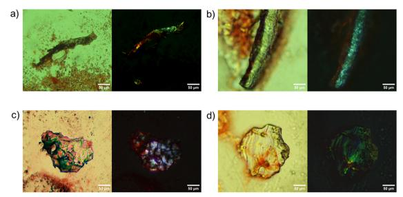
Fig. 3 Polarized optical microscopy. Images of a-K2 (a), c-K2 (b), q-K2 (c) and t-K2 (d) dried onto a glass slide and stained with Congo red solution. Films are observed using a Opteck microscope under bright-field illumination (left) and between crossed polars (right).
