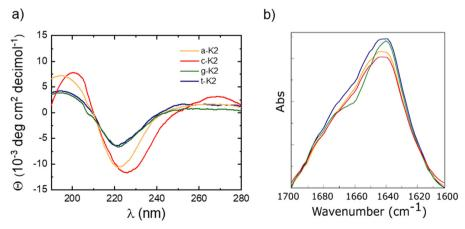
Fig. 2 Secondary structural characterization of peptides at the concentration of 0.1 wt%: (a) CD spectra recorded between 280 and 190 nm and (b) FT-IR amide I deconvolution profiles. a-K2 (orange line), c-K2 (red line), g-K2 (green line) and t-K2 (blue line)
