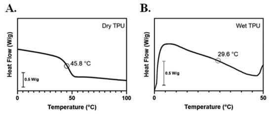
Fig. 2 Thermal characterization revealed that the glass transition temperature  $(T_0)$  of the thermoplastic polyurethane (TPU) decreased when hydrated. Differential scanning calorimetry (DSC) curves following second heating cycle of (A) dry and first heating cycle of (B) wet shape memory MM-4520 thermoplastic polyurethane
