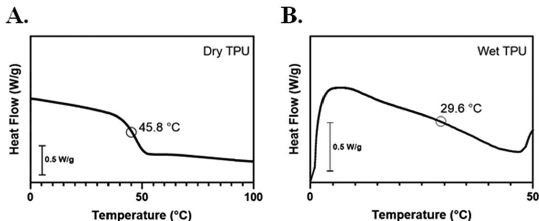
Fig. 2 Thermal characterization revealed that the glass transition temperature ( $T_g$ ) of the thermoplastic polyurethane (TPU) decreased when hydrated. Differential scanning calorimetry (DSC) curves following second heating cycle of (A) dry and first heating cycle of (B) wet shape memory MM-4520 thermoplastic polyurethane.
