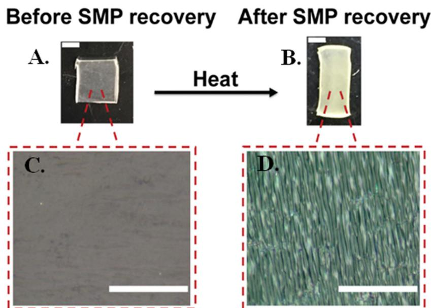
**Fig. 3** Macroscopic change in opacity of the shape memory polymer (SMP) surface induced a microscopic wrinkle formation following shape recovery. (A) Photo of 45% pre-strained SMP spin-coated with silk fibroin (SF) at 3000 rpm and then treated in methanol solution before and (B) after SMP recovery (scale bars = 5 mm). (C) Optical micrograph of 45% pre-strained SMP coated with SF and treated with methanol before and (D) after SMP recovery (scale bars = 20  $\mu\text{m}$ ).
