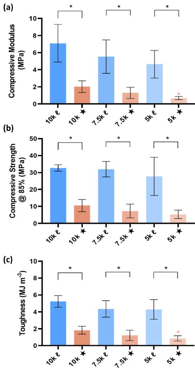
Fig. 5 Compressive (a) modulus, (b) strength (at  $\epsilon = 85\%$ ), and (c) toughness of scaffolds. "Black \*"  $p < 0.05$  comparing *linear*- and *star*- scaffolds of same  $M_n$ . "Blue \*"  $p < 0.05$  versus 10k $\ell$ . "Pink \*"  $p < 0.05$  versus 10k $\star$ .
