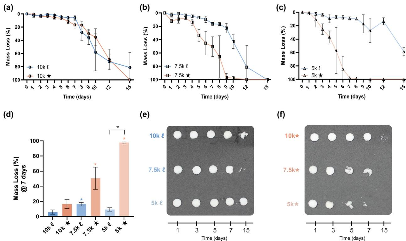
Fig. 4 Base-catalyzed (0.1 M NaOH, 37 °C) degradation studies of scaffolds prepared from (a) 10  $\text{kg mol}^{-1}$ , (b) 7.5  $\text{kg mol}^{-1}$ , and (c) 5  $\text{kg mol}^{-1}$  macromers. (d) Mass loss at 7 days. (e) and (f) Representative photos of specimens at different timepoints. "Black \*\*"  $p < 0.05$  comparing *linear*- and *star*- scaffolds of same  $M_n$ . "Blue \*\*"  $p < 0.05$  versus 10kℓ. "Pink \*\*"  $p < 0.05$  versus 10k★.
