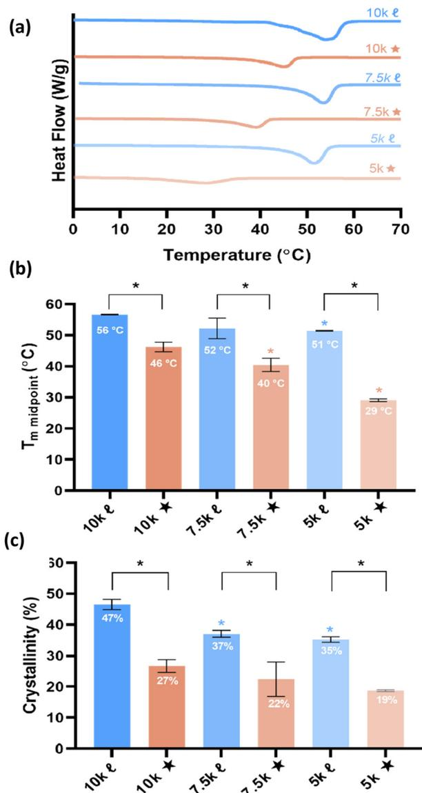
Fig. 2 (a) Representative DSC thermograph of scaffolds. (b)  $T_m$  values. (c) % Crystallinity values. “Black\*”  $p < 0.05$  comparing linear- and star- scaffolds of same  $M_n$ . “Blue\*”  $p < 0.05$  versus 10k/. “Pink\*”  $p < 0.05$  versus 10k★.
