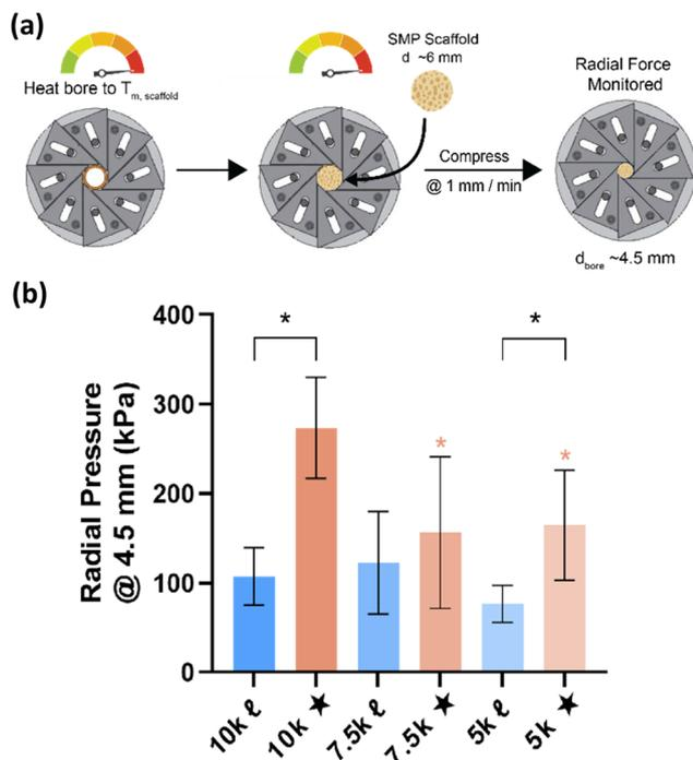
Fig. 3 (a) Protocol to measure, and (b) radial pressure exerted by scaffold specimens at designated  $T_m$ . "Black \*\*"  $p < 0.05$  comparing *linear*- and *star*- scaffolds of same  $M_n$ . "Blue \*\*"  $p < 0.05$  versus 10kℓ. "Pink \*\*"  $p < 0.05$  versus 10k★.
