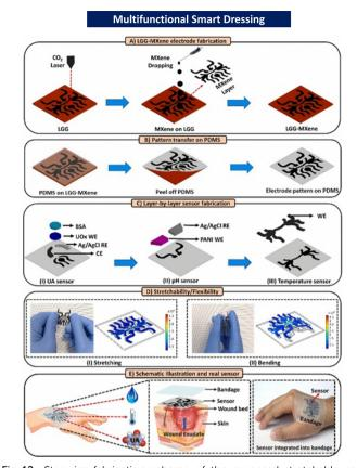
Fig. 12 Stepwise fabrication scheme of the proposed stretchable and flexible smart bandage with an integrated multifunctional sensor. MXene (a novel class of 2D multilayered nanosheets); LGG-MXene (laser-guided graphene-MXene); PDM (polydimethylsiloxane); BSA (bovine serum albumin); WE (LGG-MXene/PDMS); CE (LGG-MXene/PDMS); RE (Ag/AgCl); UOx (uricase enzyme); and PANI (pH-sensitive membrane). Reproduced from ref. 30 with permission from [Elsevier], 2023.
