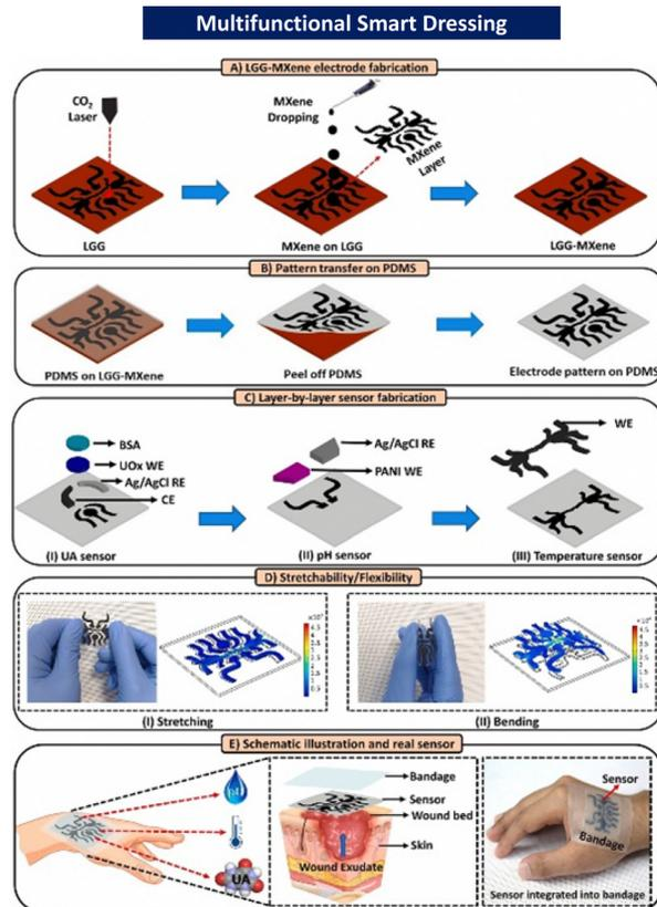
Fig. 12 Stepwise fabrication scheme of the proposed stretchable and flexible smart bandage with an integrated multifunctional sensor. MXene (a novel class of 2D multilayered nanosheets); LGG-MXene (laser-guided graphene-MXene); PDM (polydimethylsiloxane); BSA (bovine serum albumin); WE (LGG-MXene/PDMS); CE (LGG-MXene/PDMS); RE (Ag/AgCl); UOx (uricase enzyme); and PANI (pH-sensitive membrane). Reproduced from ref. 30 with permission from [Elsevier], 2023.
