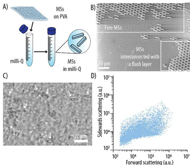
**Fig. 3** (A) Schematic illustration of the harvesting of the microgel shapes (MSs) from the polyvinyl alcohol (PVA) substrates by dissolution in Milli-Q. (B) Scanning electron microscopy micrograph of the MSs and MSs interconnected with a flash layer on the PVA substrate. (C) Bright field image of the MS suspensions after filtration showing the individual rod-like MS. (D) Flow cytometry dot plot of the MSs.
