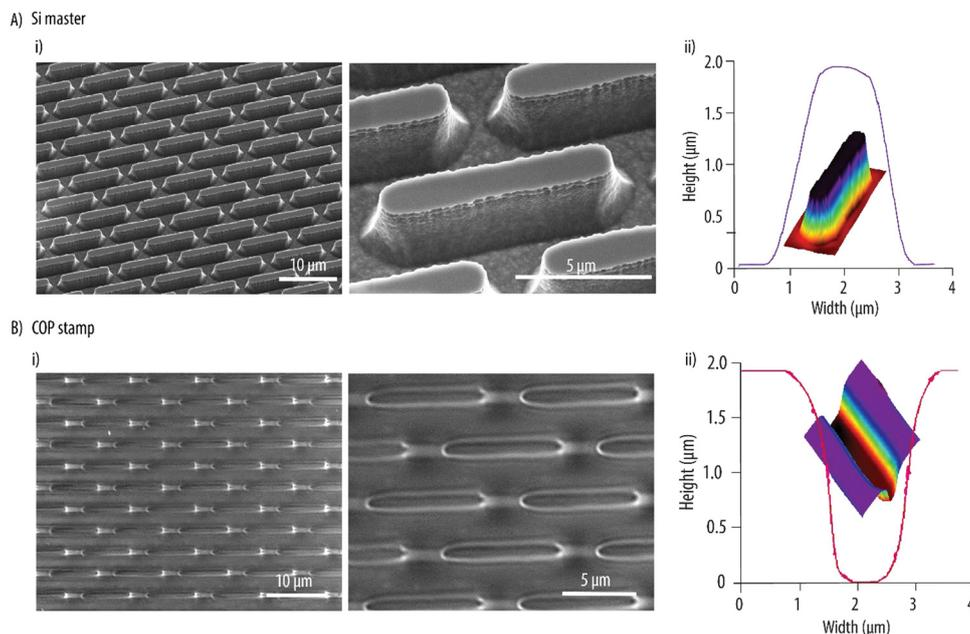
**Fig. 1** (A) (i) SEM micrographs and (ii) optical profilometer measurements with cross-sectional profile and 3D rendering of rod-like micro-structures in Si. (B) (i) SEM micrographs and (ii) optical profilometer measurements with cross-sectional profile and 3D rendering of the corresponding microwells in a cyclo olefin polymer (COP) stamp.
