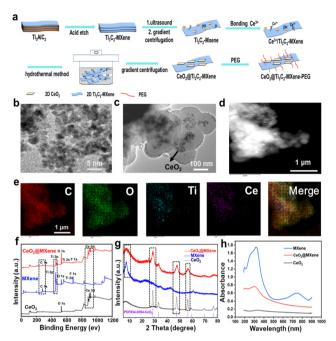
Fig. 1 (a) Schematic diagram of the preparation of the CeO<sub>2</sub>@MXene heterojunction. (b) TEM image of CeO<sub>2</sub>. (c) TEM image of CeO<sub>2</sub>@MXene. (d) and (e) CeO<sub>2</sub>@MXene-STEM images and the corresponding elemental mapping images for C, O, Ti, and Ce. (f) X-ray photoelectron spectroscopy images of CeO<sub>2</sub>/MXene/CeO<sub>2</sub>@MXene. (g) XRD pattern of CeO<sub>2</sub>/MXene/ CeO2@MXene. (h) Absorption spectra of CeO2/MXene/CeO2@MXene.
