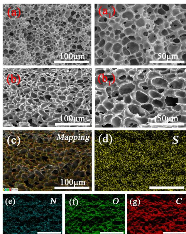
Fig. 3 The SEM images of the PAM hydrogel (a) and (a<sub>1</sub>), the PAPP hydrogel (b) and (b<sub>1</sub>), and the corresponding EDX element mapping of the PAPP hydrogel (c), including sulfur (d), nitrogen (e), oxygen (f), and carbon (g).
