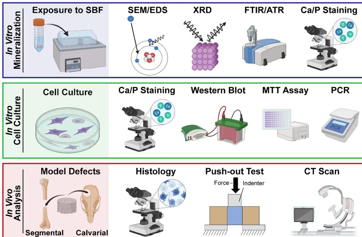
Fig. 4 Generalized methods for assessing scaffold bioactivity: (top) acellular mineralization via exposure to SBF, characterization of HAp mineralization, (middle) cell culture, and (bottom) *in vivo* analyses using bone defect models.
