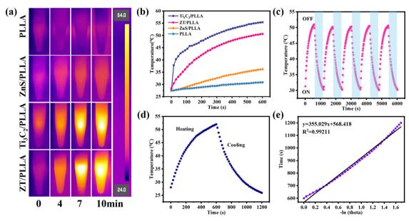
Fig. 4 Photothermal images (a) and curves (b) of the composite scaffolds under NIR light for different irradiation times. (c) Thermal cycle curves of the ZT/PLLA scaffold. (d) Single temperature rising and cooling curve of the ZT/PLLA scaffold. (e) Regression curve of the ZT/PLLA scaffold.
