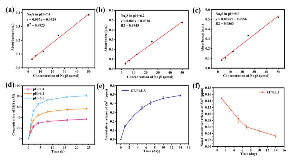
Fig. 5 (a)-(c) Na<sub>2</sub>S standard curve at different pH. (d) Cumulative release of H<sub>2</sub>S at different pH. Cumulative (e) and non-cumulative (f) release curves of Zn2+ of the ZT/PLLA scaffold in PBS
