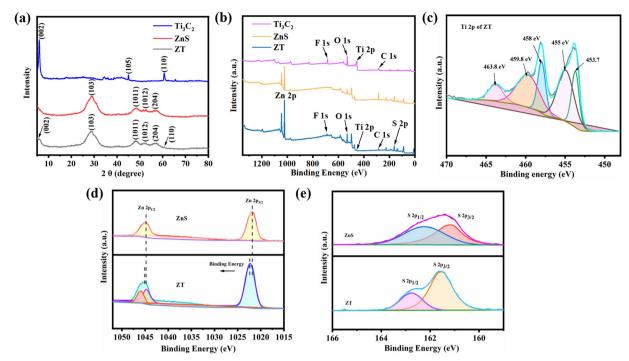
Fig. 2 XRD (a) and full XPS survey (b) spectra of ZnS, Ti<sub>3</sub>C<sub>2</sub> and ZT nanoparticles. (c) High-resolution Ti 2p XPS spectra of ZT. (d) High-resolution Zn 2p XPS spectra of ZnS and ZT. (e) High-resolution S 2p XPS spectra of ZnS and ZT.
