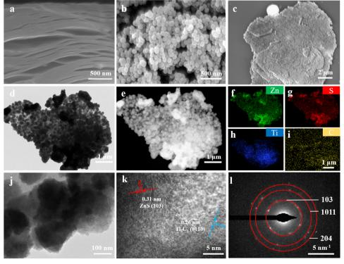
Fig. 1 SEM images of  $Ti_3C_2$  (a), ZnS (b) and ZT (c). (d) Low-resolution TEM image of ZT. Dark-field (e) and element mapping (f)—(i) of ZT. TEM (j), high-resolution TEM (k) and SAED (l) images of ZT nanoplatform.
