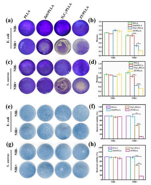
Fig. 6 E. coli (a) and S. aureus (c) biofilm crystalline violet staining after different treatments. Biofilm biomass of E. coli (b) and S. aureus (d) after different treatments. Typical photos of bacterial colonies of E. coli (e) and S. aureus (g) in different groups. Number of CFU of E. coli (f) and S. aureus (h) in different treatment groups.
