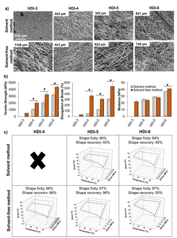
Fig. 7 (a) Scanning electron micrographs of electrospun fibers with overlaid fiber diameter (n = 10, quantified using Imagej). Scale bar applies to all images. (b) Tensile properties of fibers. n = 3, mean  $\pm$  standard deviation displayed. \*p < 0.05 between each group. (c) Dynamic mechanical analysis of fibers with corresponding shape fixity and shape recovery values (n = 1;  $\times$ : no shape memory properties were observed).
