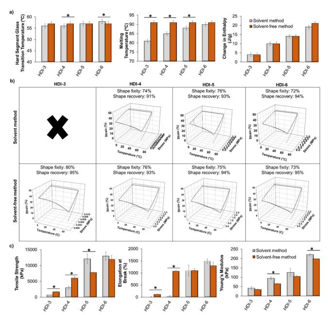
Fig. 3 Comparison of (a) thermal (n = 3), (b) shape memory  $(n = 1, \times)$  no shape memory properties were observed), and (c) tensile (n = 3) properties of polymers synthesized using solvent-based (data are from our previous work $^{32}$ ) and solvent-free methods. Mean  $\pm$  standard deviation displayed. \*p < 0.05 relative to corollary sample synthesized using solvent-based method.
