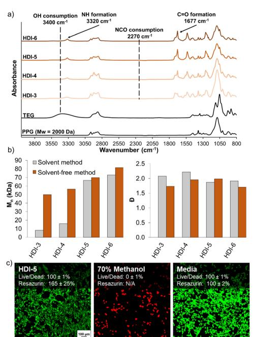
Fig. 2 (a) Characterization of synthesized segmented thermoplastic polyurethanes using Fourier transform infrared (FTIR) spectroscopy. (b) Number average molecular mass ( $M_{pr}$ , left) and polydispersity index (D, right) of polymers synthesized with and without solvent (n = 1). (c) Cytocompatibility of representative segmented thermoplastic polyurethane (HDI-5) measured using live/dead and resazurin assays (n = 3, mean  $\pm$  standard deviation displayed, scale bar applies to all images).
