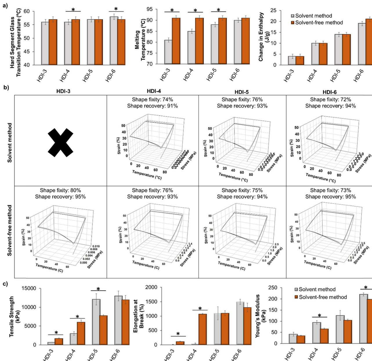
Fig. 3 Comparison of (a) thermal ( $n = 3$ ), (b) shape memory ( $n = 1$ ,  $\times$ : no shape memory properties were observed), and (c) tensile ( $n = 3$ ) properties of polymers synthesized using solvent-based (data are from our previous work<sup>32</sup>) and solvent-free methods. Mean  $\pm$  standard deviation displayed. \* $p < 0.05$  relative to corollary sample synthesized using solvent-based method.
