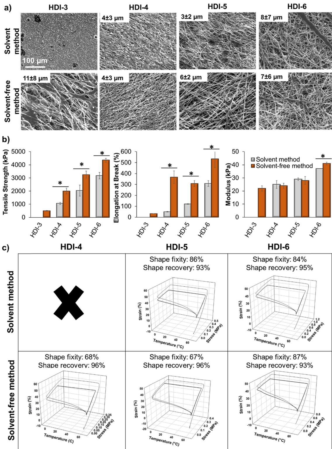
Fig. 7 (a) Scanning electron micrographs of electrospun fibers with overlaid fiber diameter ( $n = 10$ , quantified using ImageJ). Scale bar applies to all images. (b) Tensile properties of fibers.  $n = 3$ , mean  $\pm$  standard deviation displayed. \* $p < 0.05$  between each group. (c) Dynamic mechanical analysis of fibers with corresponding shape fixity and shape recovery values ( $n = 1$ ; X: no shape memory properties were observed).
