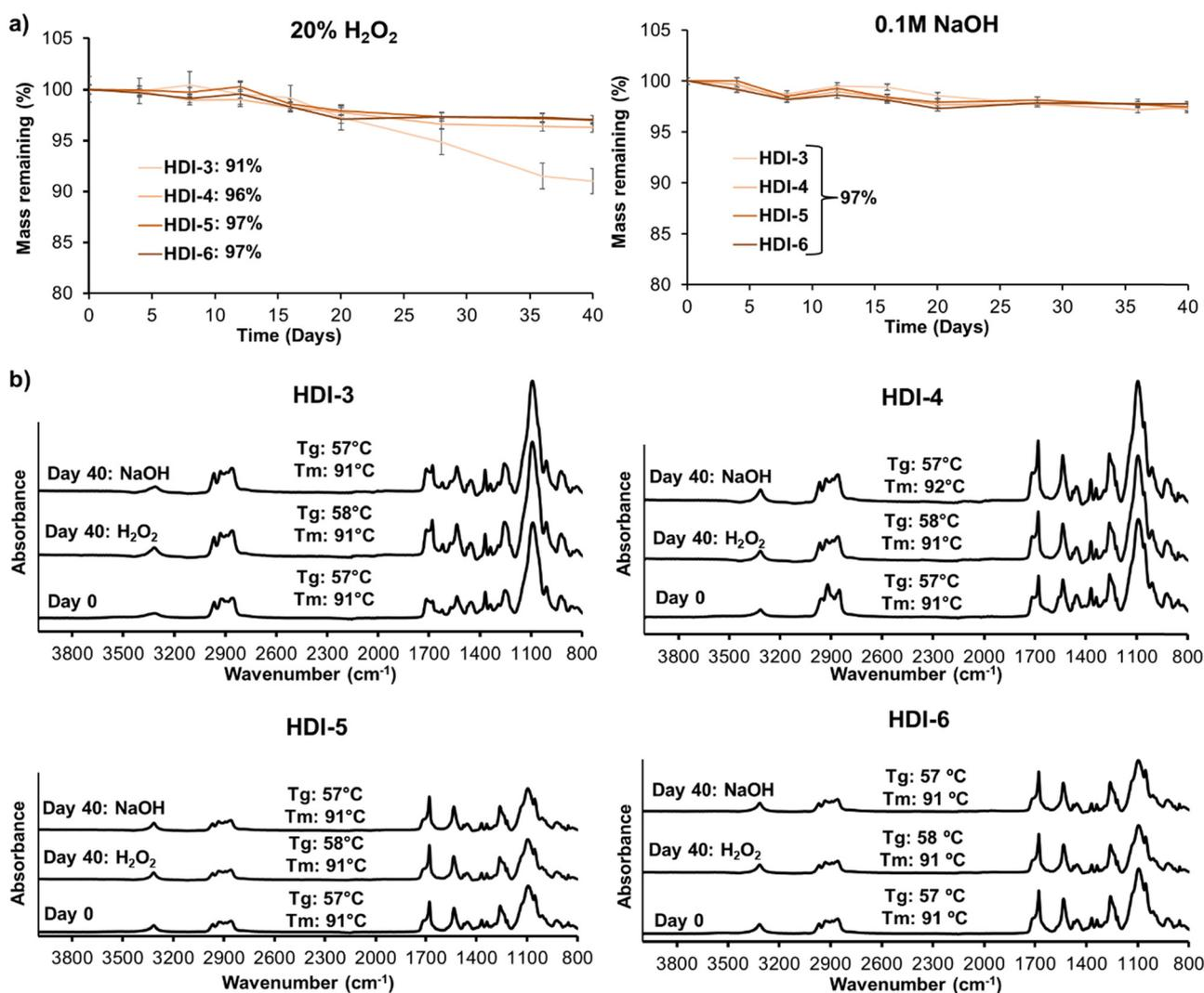
Fig. 4 (a) Mass remaining of segmented thermoplastic polyurethanes synthesized by solvent free method in (left) 20% H<sub>2</sub>O<sub>2</sub> and (right) 0.1M NaOH over 40 days.  $p > 0.05$  between day 0 and 40 for each formulation and between all formulations at day 40. (b) FTIR spectra and corresponding  $T_g$  and  $T_m$  ( $n = 1$ ) at 0 and 40 days of incubation in hydrolytic and oxidative media for HDI-3, HDI-4, HDI-5, and HDI-6.
