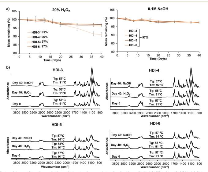
Fig. 4 (a) Mass remaining of segmented thermoplastic polyurethanes synthesized by solvent free method in (left) 20% H<sub>2</sub>O<sub>2</sub> and (right) 0.1 M NaOH over 40 days. p > 0.05 between day 0 and 40 for each formulation and between all formulations at day 40. (b) FTIR spectra and corresponding  $T_{\rm q}$  and  $T_{\rm m}$ (n = 1) at 0 and 40 days of incubation in hydrolytic and oxidative media for HDI-3, HDI-4, HDI-5, and HDI-6.
