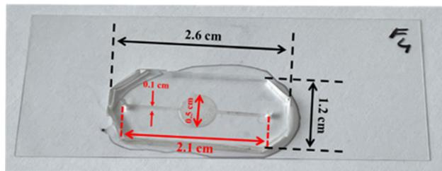
Fig. 1 The as-developed final microfluidic plasmonic chip.
