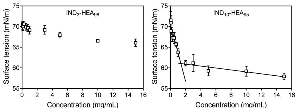
Fig. 5 Surface tension measurements of representative copolymers  $\text{IND}_3$ - $b$ - $\text{HEA}_{98}$  and  $\text{IND}_{10}$ - $b$ - $\text{HEA}_{95}$  carried out in water by pendant drop method.<sup>36</sup>
