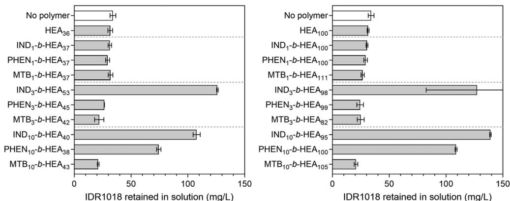
Fig. 7 The concentration of IDR 1018 remaining in a solution after incubation in aggregation conditions (100 mM phosphate buffer, pH 7.2) for 5 h without and with synthesised copolymers at 1 : 1 molar ratio; the initial concentration of the peptide was 0.153 mg mL<sup>-1</sup>. Higher values in the graph correspond to better protein stabilisation and hence reduced aggregation.
