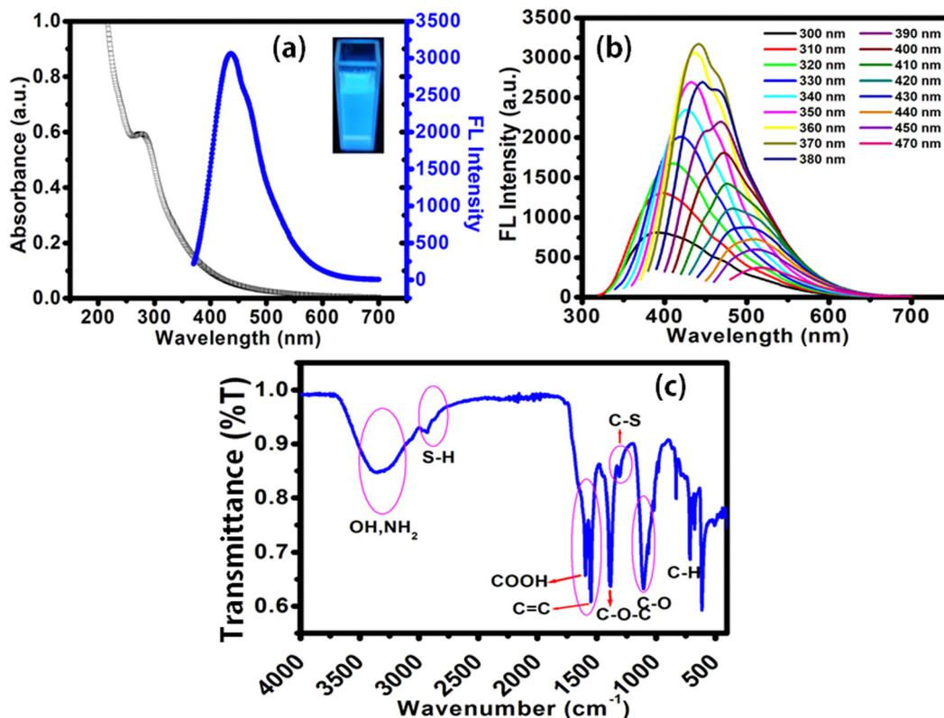
**Fig. 1** (a) Absorption and FL spectra of OCDs excited at 360 nm. Inset: Strong blue FL of OCD solution observed by the naked eyes under 365 nm UV lamp illumination. (b) FL spectra of OCDs excited at different wavelengths ranging from 300 nm to 470 nm and (c) FT-IR spectra of OCDs.
