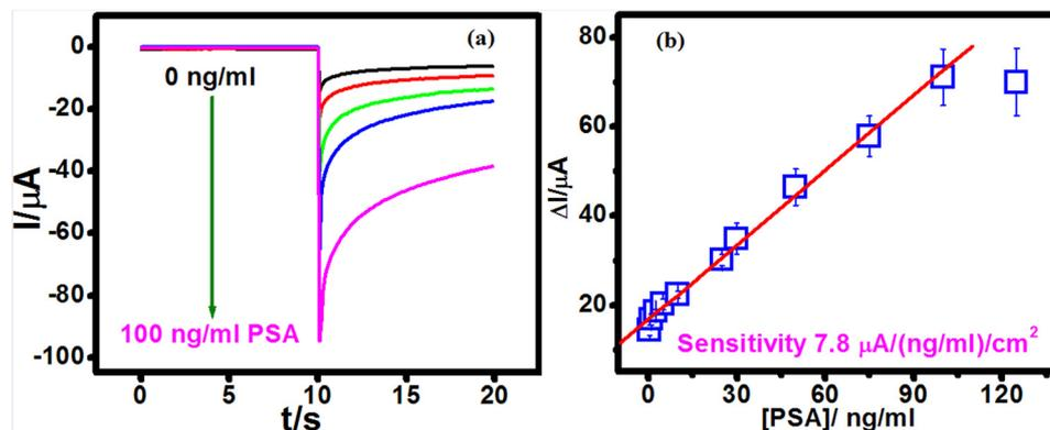
Fig. 6 (a) Amperometric curves of  $\text{OCD@}^{\text{PSA}}\text{Ab}_2$  detection probe-based PSA biosensor in the presence of 3 mM HQ and 4.5 mM  $\text{H}_2\text{O}_2$  at different concentrations of PSA and (b) the calibration plot for the  $\text{OCD@}^{\text{PSA}}\text{Ab}_{\text{HRP}}$ -based PSA biosensor.
