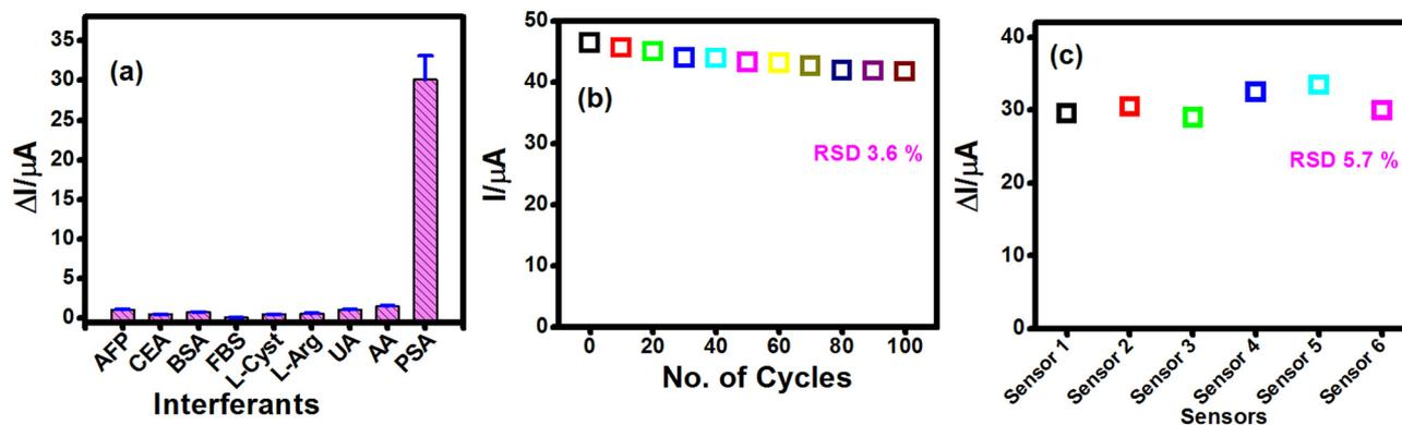
Fig. 7 (a) Specificity studies of the biosensor in the presence of AFP, CEA, BSA, FBS, L-cysteine, L-arginine, AA, and UA; (b) cathodic current obtained from  $\text{PSAAb}_{\text{cap}}$ -bound immobilization matrix during cyclic voltammetry for 100 cycles in PBS containing HQ, and (c) the response of 6 different biosensors to  $10 \text{ ng ml}^{-1}$  of PSA.
