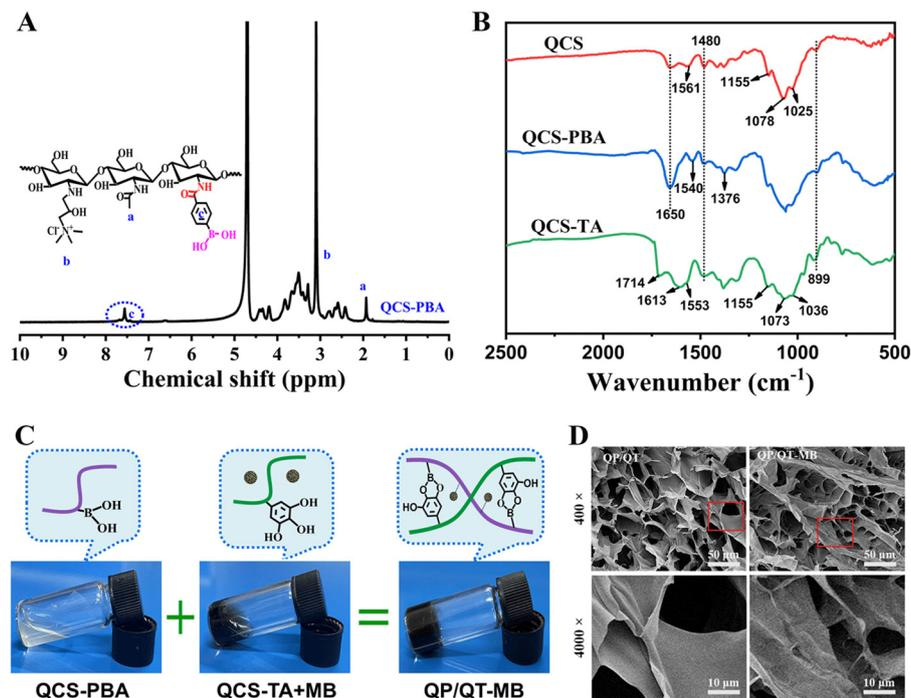
Fig. 2 (A)  $^1\text{H}$  NMR spectrum of QCS-PBA. (B) FTIR spectra of QCS, QCS-PBA, and QCS-TA. (C) The gelation process of QP/QT-MB hydrogel. (D) SEM images of QP/QT and QP/QT-MB hydrogels at different magnifications.
