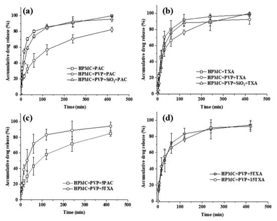
Fig. 8 In vitro drug release data of SSE 3D printed tablets of (a) PAC-loaded tablets, (b) TXA-loaded tablets, (c) the influence of API type, and (d) the influence of API concentration.
