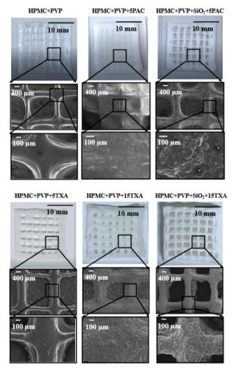
Fig. 6 Physical appearances and SEM images of dried 3D printed tablets of HPMC + PVP, HPMC + PVP + 5PAC, HPMC + PVP + SiO<sub>2</sub> + 5PAC, HPMC + PVP + 5TXA, and HPMC + PVP + 15TXA, HPMC + PVP + SiO<sub>2</sub> + 15TXA.
