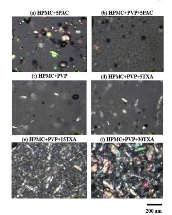
Fig. 2 The polarized light microscopy images of the inks with (a) HPMC + 5PAC, (b) HPMC + PVP + 5PAC, (c) HPMC + PVP, (d) HPMC + PVP + 5TXA, (e) HPMC + PVP + 15TXA and (f) HPMC + PVP + 30TXA.
