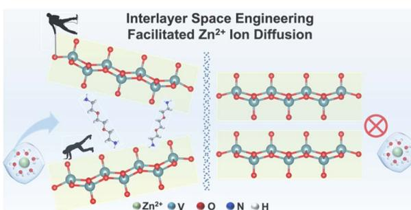
**A layer separated  $V_2O_5$ -PEG-amine hybrid cathode material for high capacity zinc-ion batteries**
