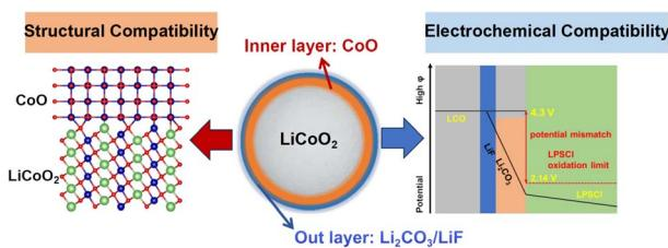
**Janus *in situ* formed CoO/Li<sub>2</sub>CO<sub>3</sub>/LiF interlayer between LiCoO<sub>2</sub> and Li<sub>6</sub>PS<sub>5</sub>Cl solid electrolytes boosting the 4.5 V performance of sulfide-based all-solid-state batteries**
