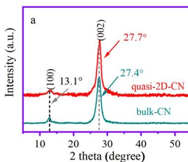
Fig. 4 (a) XRD patterns of bulk-CN and quasi-2D-CN.
