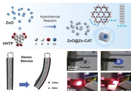
**Novel two-dimensional conductive metal–organic framework-based heterostructures for high-performance electro-ionic soft actuators**
