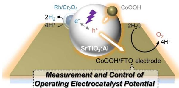
**Operando measurement of electrocatalyst potential on particulate photocatalysts for overall water splitting**
