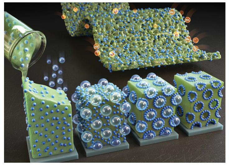
Highlighting a study on composite gel polymer electrolytes for sodium metal batteries prepared via breath-figure self-assembly by a group of researchers led by Prof. Jimin Shim from Seoul National University.
