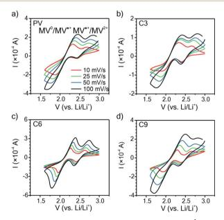
Fig. 3 Cyclic voltammograms at 10, 25, 50, and 100 mV s $^{-1}$ for (a) PV, (b) C3, (c) C6, and (d) C9 thin films on ITO-coated glass as working electrodes in a three-electrode beaker cell configuration. The supporting electrolyte was 0.5 M LiCl in GBL. Lithium metal was used as counter and reference electrodes.
