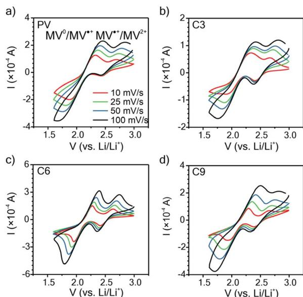
Fig. 3 Cyclic voltammograms at 10, 25, 50, and 100 mV s<sup>-1</sup> for (a) PV, (b) C3, (c) C6, and (d) C9 thin films on ITO-coated glass as working electrodes in a three-electrode beaker cell configuration. The supporting electrolyte was 0.5 M LiCl in GBL. Lithium metal was used as counter and reference electrodes.
