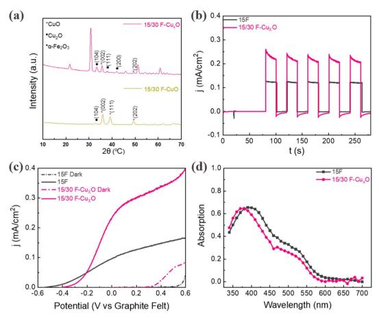
Fig. 2 (a) XRD of different photoelectrodes; (b) photoresponse behavior for 15/30F-Cu<sub>x</sub>O and 15F with 20 s light on-off; (c) linear sweep voltammetry curve for 15/30F-Cu<sub>x</sub>O and 15F both under 1 sun illumination and dark; (d) UV-vis absorption spectrum of 15/30F-Cu<sub>x</sub>O and 15F.
