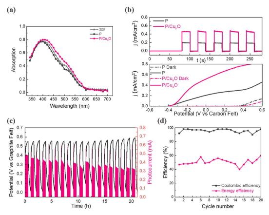
Fig. 4 (a) UV-vis absorption spectrum of nanostructures and 30F; (b) photoresponse behavior for  $P/Cu_xO$  and P with 20 s light on-off; linear sweep voltammetry curve for  $P/Cu_xO$  and P both under 1 sun illumination and dark; (c) representative photocharge-discharge cycling behavior with a cut-off potential set to 0-0.58 V and unbiased photocurrent using  $P/Cu_xO$  photoanode; (d) coulombic and energy efficiency of photocharge/discharge curve.
