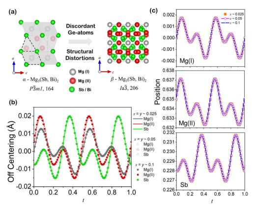
Fig. 5 (a) Schematic depicting trigonal and superionic phase transitions. The tetrahedral and octahedral polyhedra are highlighted in the trigonal phase. (b) Evaluated off-centering for Mg(ı), Mg(ıı) and Sb atoms for varying compositions. (c) Corresponding positional modulations of the atomic coordinates of Mg(ı)  $\sim$  (0, 0, 0), Mg(ıı)  $\sim$  (1/3, 2/3, 0.634), and Sb  $\sim$  (1/3, 2/3, 0.229) atoms plotted as a function of the fourth superspace coordinate (t).
