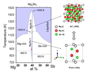
Fig. 1 The Mg-Sb phase diagram near Mg<sub>3</sub>Sb<sub>2</sub> indicating the phase transformation of  $\alpha$ -Mg<sub>3</sub>Sb<sub>2</sub> ( $P\bar{3}m1$ , 164)  $\leftrightarrow$   $\beta$ -Mg<sub>3</sub>Sb<sub>2</sub> ( $Ia\bar{3}$ , 206).<sup>16-18</sup>
