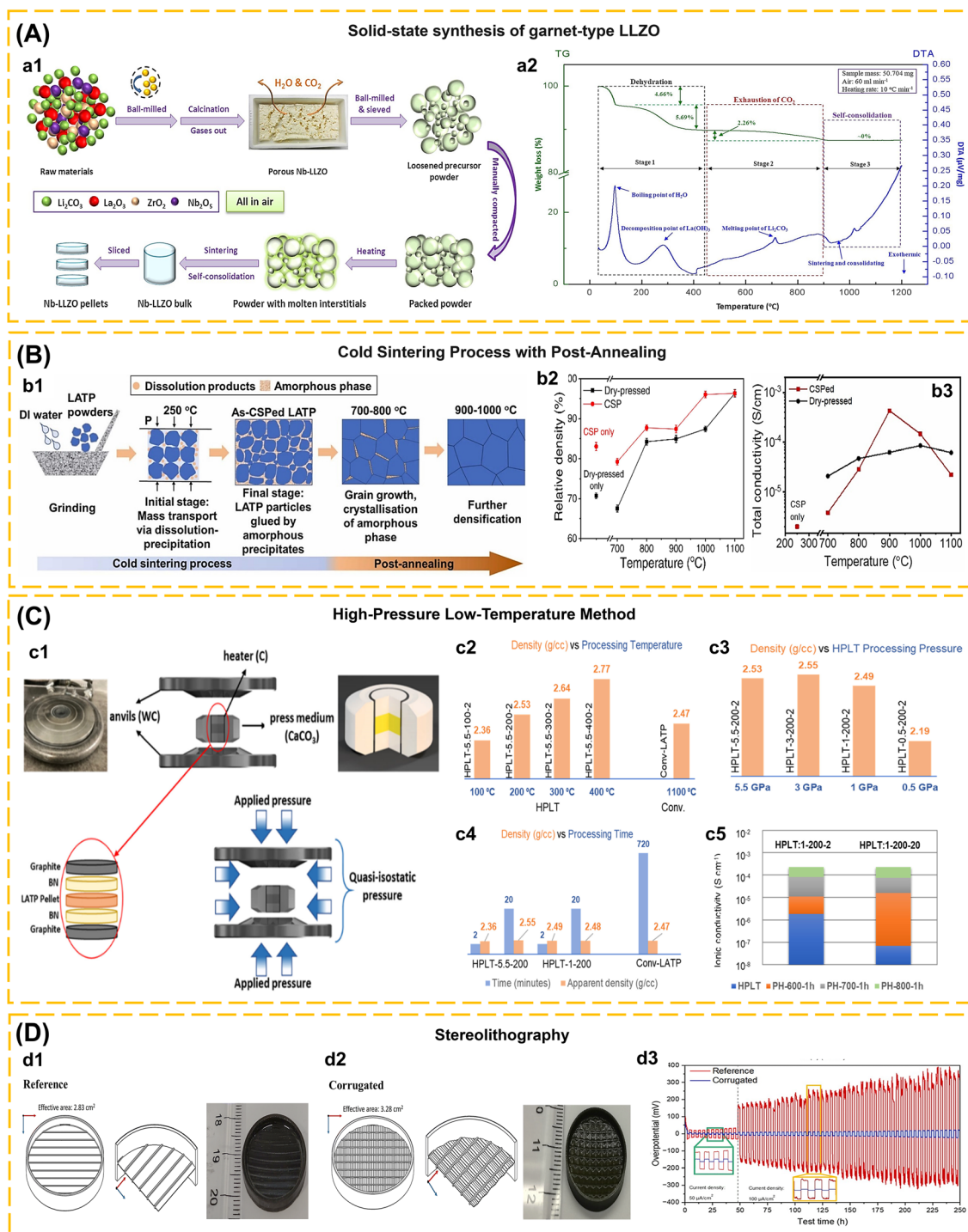
Fig. 13 (A) (a1) Schematic illustration for the preparation of Nb-LLZO pellets by self-consolidation method. (a2) TG/DTA curves of the precursor 060Nb-LLZO powder before sintering. Reproduced with permission from ref. 136. Copyright 2018, Elsevier. (B) (b1) Schematic illustration of the microstructure evolution in LATP ceramics during CSP and subsequent post-annealing. (b2) Effect of annealing temperatures on the relative density of LATP samples produced by CSP and dry-pressing. All samples were annealed for 1 h. (b3) Total ionic conductivity (measured at room temperature) of the CSPed and dry-pressed LATP samples as a function of annealing temperature. Reproduced with permission from ref. 83. Copyright 2023, Elsevier. (C) (c1) The schematic representation of components for the HPLT technique. Density of LATP pellets densified by HPLT processing and conventional sintering. From top to down: (c2) LATP density vs. HPLT processing temperature for pellets processed at 5.5 GPa and 2 minutes compared to conventional sintering, (c3) LATP density vs. HPLT processing pressure for pellets processed at 200^{\circ}\text{C} and for 2 min, (c4) LATP density vs. HPLT processing time for pellets processed at 200^{\circ}\text{C} and under high (5.5 GPa) and low (1 GPa) processing pressures compared to conventional sintering conditions. (c5) Evolution of Li-ion conductivity with increase in PH temperature: HPLT-1-200-2 (b) pellet:
