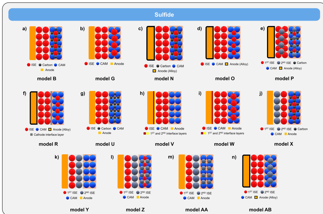
Fig. 23 Current models of ASSBs assembly for sulfide-based ISEs: (a) model B, (b) model G, (c) model N, (d) model O, (e) model P, (f) model R, (g) model U, (h) model V, (i) model W, (j) model X, (k) model Y, (l) model Z, (m) model AA, (n) model AB.
