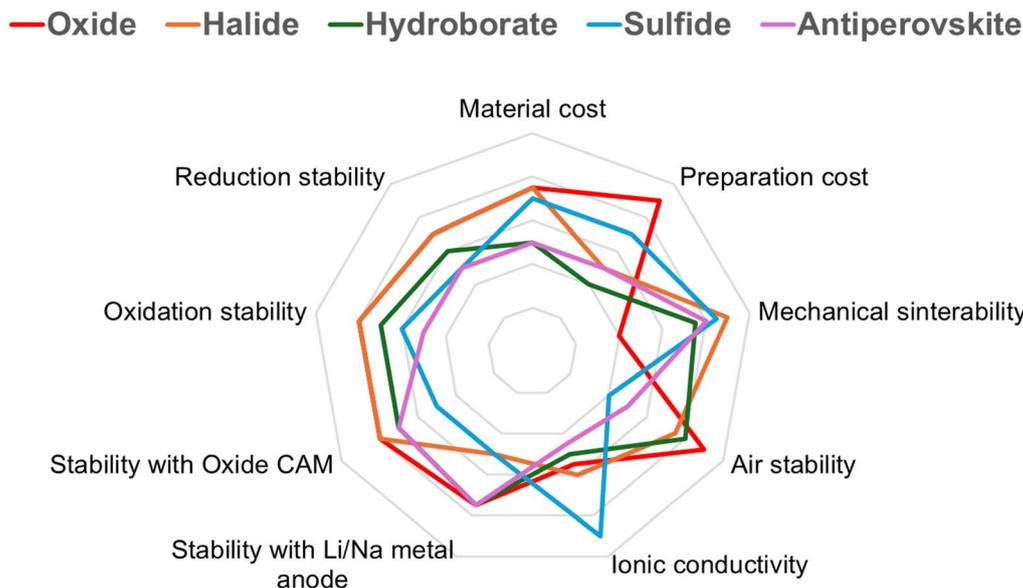
Fig. 24 Comparison of the properties of Na/Li-based ISEs.
