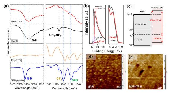
Fig. 4 FTIR spectra of the TFSI powder, PbI<sub>2</sub>-TFSI mixture, MAPI film and MAPI/TFSI film in a comparative presentation (a). UPS spectra (b), schematic diagram of the relative energy level positions (c), and Kelvin probe AFM images (d and e) of FTO/TiO<sub>2</sub>/MAPI and FTO/TiO<sub>2</sub>/MAPI/TFSI films of the corresponding devices
