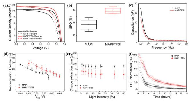
Fig. 5 J-V characteristics under forward (dashed lines) and reverse scan (a), statistical analysis of the SPO (b), capacitance-frequency plots (c), recombination lifetime against  $V_{OC}$  (d), charge extraction time under different illuminations (e) and PCE stability under light stress (ISOS-L-1) (f), for planar PSCs based on MAPI films, with and without TFSI passivation
