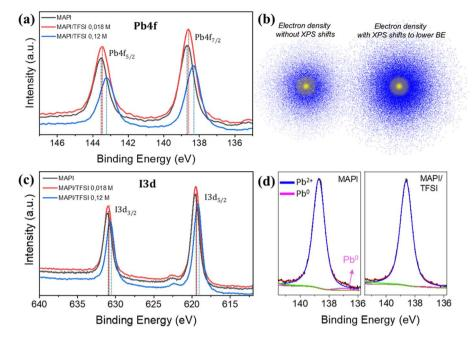
Fig. 3 Pb4f XPS spectra of MAPI and MAPI/TFSI films (a), schematic illustration of the correlation between XPS shifts and an atom's electron density (b), I3d XPS spectra (c) and Pb4f XPS spectra focused on 4f7/2 peaks (d) of MAPI and MAPI/TFSI films.
