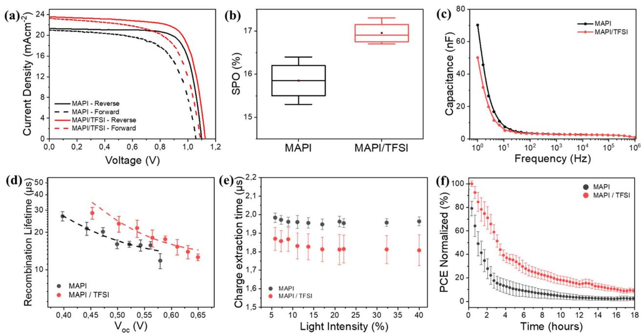
Fig. 5  $J$ - $V$  characteristics under forward (dashed lines) and reverse scan (a), statistical analysis of the SPO (b), capacitance–frequency plots (c), recombination lifetime against  $V_{OC}$  (d), charge extraction time under different illuminations (e) and PCE stability under light stress (ISOS-L-1) (f), for planar PSCs based on MAPI films, with and without TFSI passivation.
