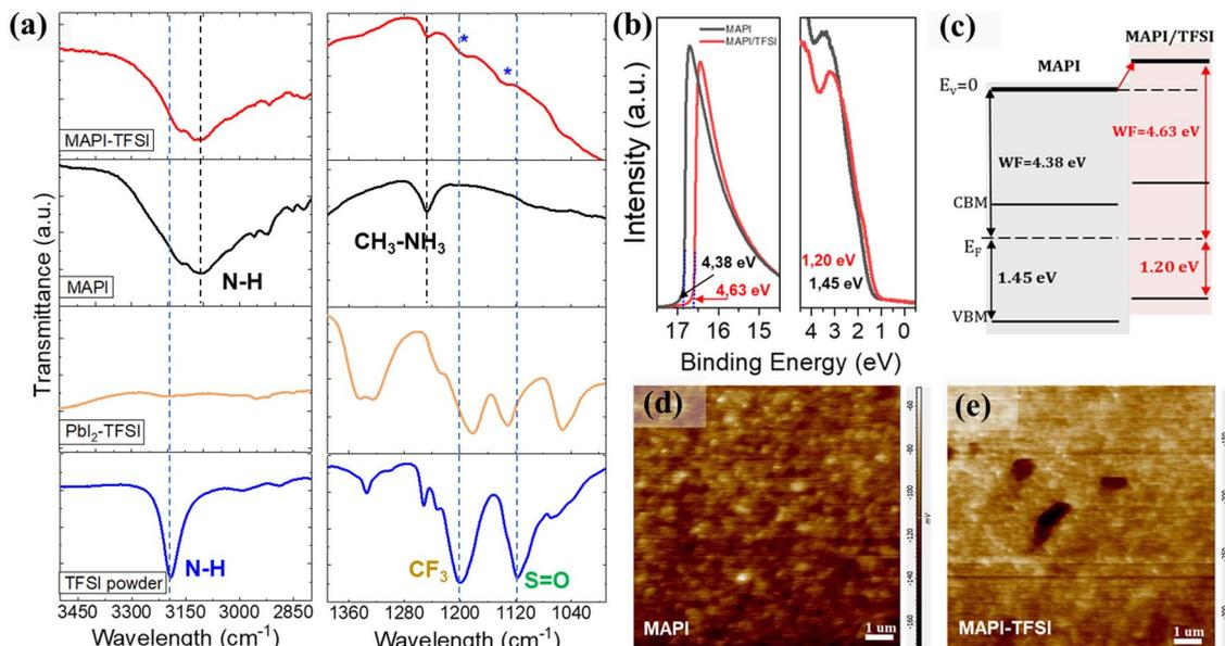
Fig. 4 FTIR spectra of the TFSI powder, Pbl<sub>2</sub>-TFSI mixture, MAPI film and MAPI/TFSI film in a comparative presentation (a). UPS spectra (b), schematic diagram of the relative energy level positions (c), and Kelvin probe AFM images (d and e) of FTO/TiO<sub>2</sub>/MAPI and FTO/TiO<sub>2</sub>/MAPI/TFSI films of the corresponding devices.
