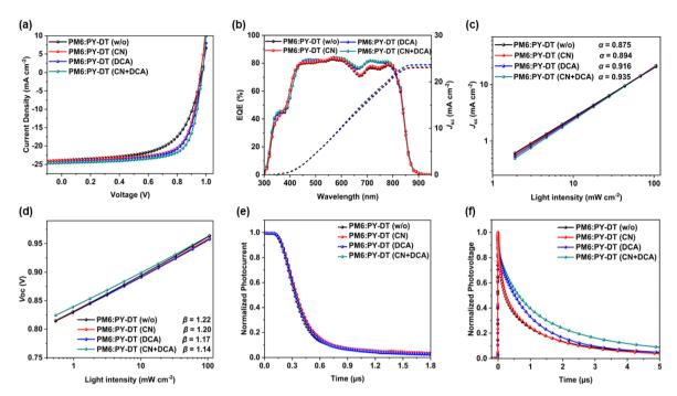
Fig. 2 (a) J-V characteristics and (b) EQE spectra and integrated  $J_{sc}$  of PM6:PY-DT fabricated under various conditions. (c)  $J_{sc}$  vs. light intensity and (d)  $V_{oc}$  vs. light intensity. (e) TPC and (f) TPV of PM6:PY-DT fabricated under various conditions.
